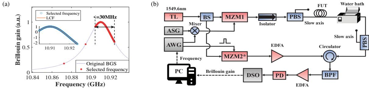
Fig. 1: (a) Working principle of the proposed scheme; (b) Experimental setup. TL: tunable laser, AWG: arbitrary waveform generator, ASG: analog signal generator, BS: beam splitter, MZM: Mach-Zehnder modulator (\*: high extinction ratio), EDFA: Erbium-doped fiber amplifier, PBS: polarization beam splitter, FUT: fiber under test, BPF: bandpass filter, PD: photodetector, DSO: digital storage oscilloscope, PC: personal computer.
