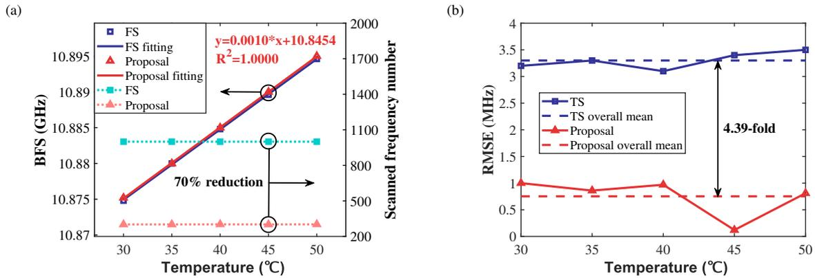
Fig. 2: (a) BFS-temperature curve and average scanned frequency number under different temperatures; (b) BFS estimation RMSE over TS scheme under different temperatures.
