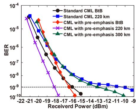
Fig. 6: BER performances for the CML signals with and without pre-emphasis.
