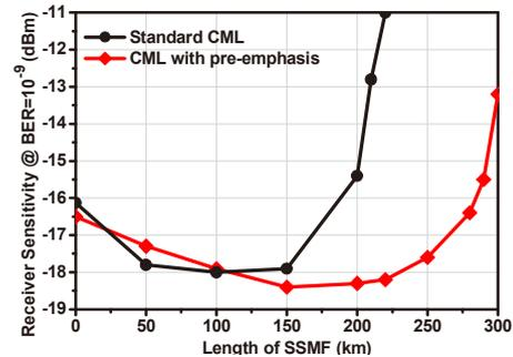
Fig. 5: Receiver sensitivities for the standard CML signal without pre-emphasis and the CML signal with pre-emphasis after various lengths of SSMF.
