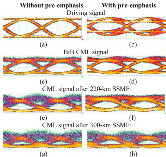
Fig. 4: Eye diagrams of the (a-b) driving signal, (c-d) BtB CML signal, (e-f) CML signal after 220-km SSMF, and (g-h) CML signal after 300-km SSMF. Time scale: 20 ps/div
