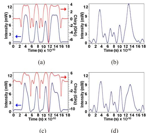
Fig. 2: Simulated intensity and chirp characteristics of (a) BTB standard CML signal, (b) standard CML signal after 300-km SSMF, (c) BTB CML signal with pre-emphasis, and (d) CML signal with pre-emphasis after 300-km SSMF with an input bit sequence of "0011001001011100".
