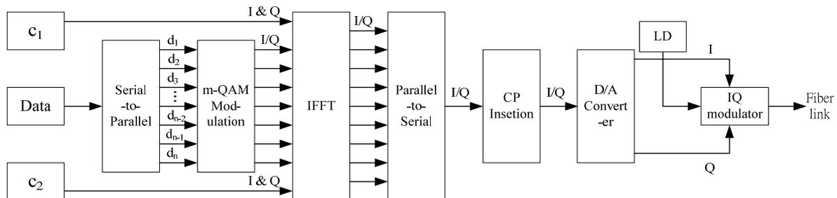
**Fig. 1:** The block diagram of the proposed CO-OFDM transmitter. (I&Q: inphase and quadrature phase components, IFFT: inverse fast Fourier transform, m-QAM: multilevel quadrature amplitude modulation, CP: cyclic prefix, D/A digital-to-analog, LD: laser diode)
