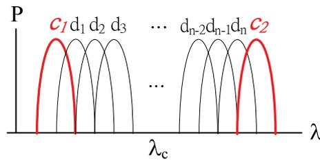
Fig. 2: Optical spectra of the generated optical OFDM signal with two optical coded label subcarriers,  $c_1$  and  $c_2$  (in red).
