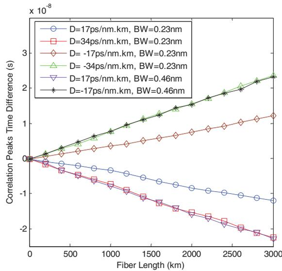
**Fig. 3:** Temporal difference of the correlation peaks between the two coded label subcarriers at different values of fiber transmission length, fiber dispersion slope and signal spectral width.
