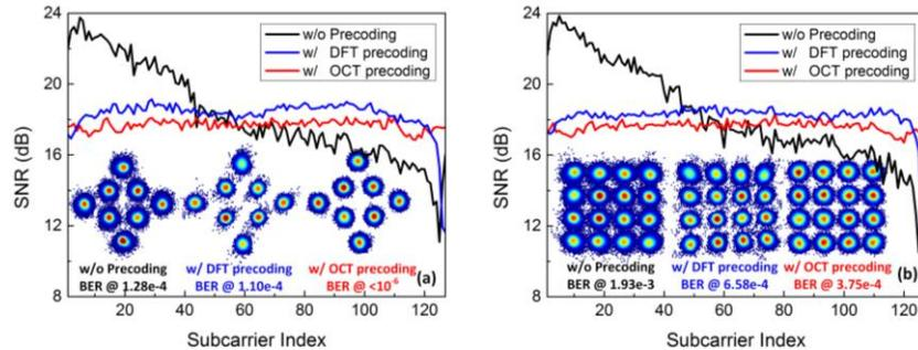
Fig. 3. Estimated SNRs and corresponding signal constellation diagrams for the system without precoding, with DFT precoding and with OCT precoding when data rate is: (a) 300 Mb/s; (b) 400 Mb/s
