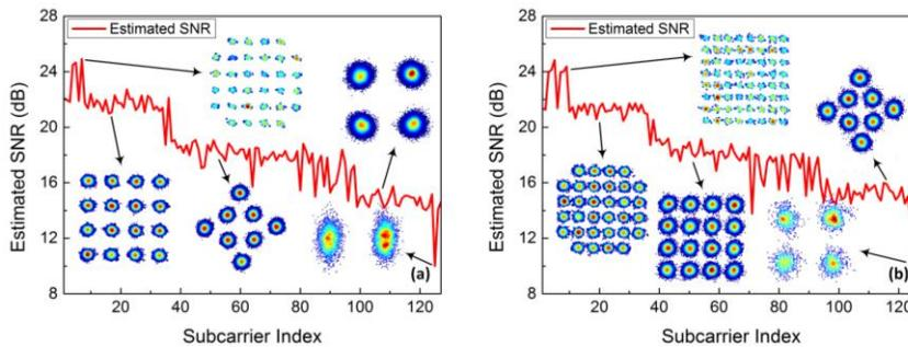
Fig. 4. Estimated SNRs and corresponding signal constellation diagrams for adaptive loading when data rate is: (a) 300 Mb/s; (b) 400 Mb/s
