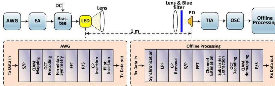
Fig. 1. Block diagram of the OCT-based VLC system. (DC: direct current; LPF: low pass filter; PD: photodiode)
