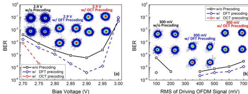
Fig. 2. Measured BERs versus (a) bias voltage of LED at  $\sim 200$  Mb/s (RMS voltage of driving signal is 100 mV) and (b) RMS voltage of driving signal (bias voltage is 2.9V). Note that the measured BER of OCT precoding scheme is below  $10^{-6}$ , and thus is not shown in Fig. 2(b).
