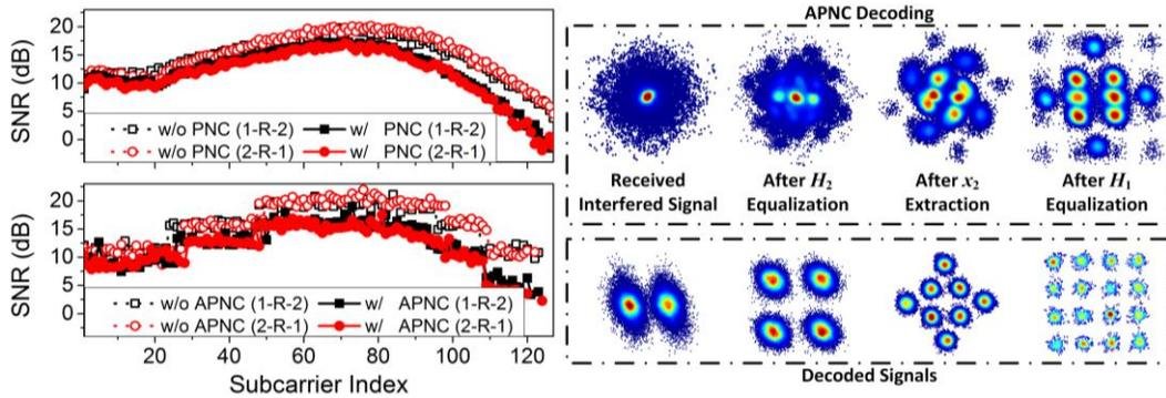
Fig. 4. SNR penalty of the system with PNC/APNC (left) and the progressing of APNC decoding and the corresponding decoded signal constellations for link 1-R-2 (right).
