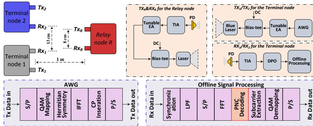
Fig. 2. Experimental setup of the OFDM-based TWR VLC network using PNC.
