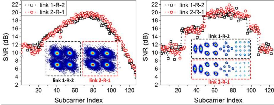
Fig. 3. SNR performance over the subcarriers: 4QAM-OFDM (left) and 4QAM-DMT (right).
