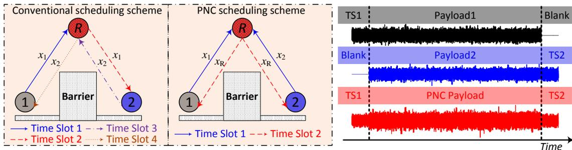
Fig. 1. Conventional scheduling and PNC scheduling (left) and packet structure for PNC over the OFDM-based TWR VLC network (right).
