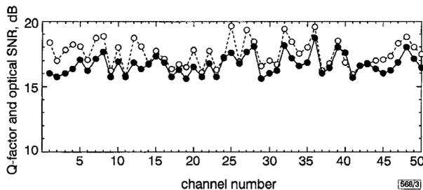
Fig. 3 Measured Q-factor and optical SNR for 50 WDM channels after 1655km transmission
