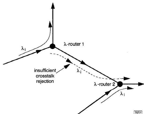
Fig. 1 Example of an optical network configuration that may induce co-channel crosstalk interference
