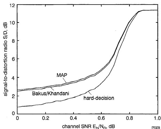
Fig. 2 Signal-to-distortion ratio against channel signal-to-noise ratio  $E_b/N_0$  for eight-dimensional vector quantiser decoded by hard-decision mapping, MAP estimator, and Bakus/Khandani decoder [4]
