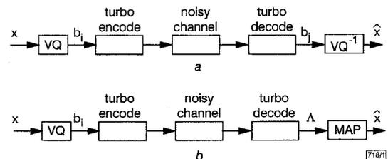
Fig. 1 Schematic diagram of communication systems for vector quantiser using turbo-codes
