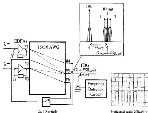
To generate the channel ID, a small portion from each of the amplifiers' outputs (through a 95:5 coupler) is fed back to its input (through a 50:50 coupler). A tunable FPF of finesse 100 with a 3-dB bandwidth of 0.7 nm is placed in between the couplers at each input fiber 1 and 3. By applying a sinusoidal voltage of 0.4 V (peak-to-peak) at 2.5 kHz to the FPF at input port 1 and an identical voltage at 3 kHz to the FPF
