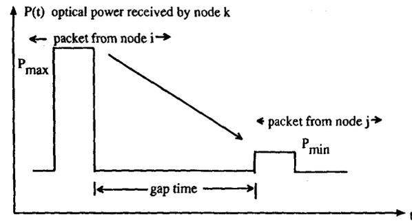
Fig. 5. The worst case for threshold shifting of a burst-mode receiver.
