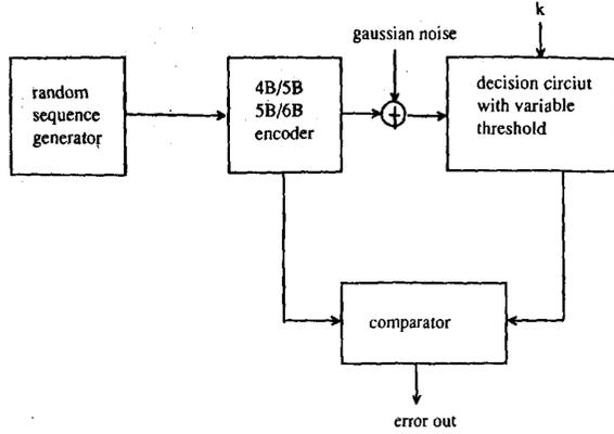
Fig. 4. Simulation experiment for burst-mode receiver with different decay parameter  $k$ .
