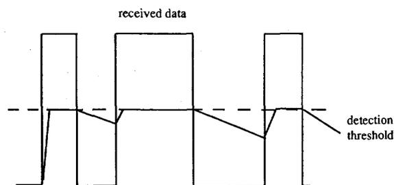
Fig. 2. The threshold of a burst-mode receiver varies according to the incoming data pattern. The dashed lines and solid lines are the thresholds for the conventional and burst-mode receivers respectively.
