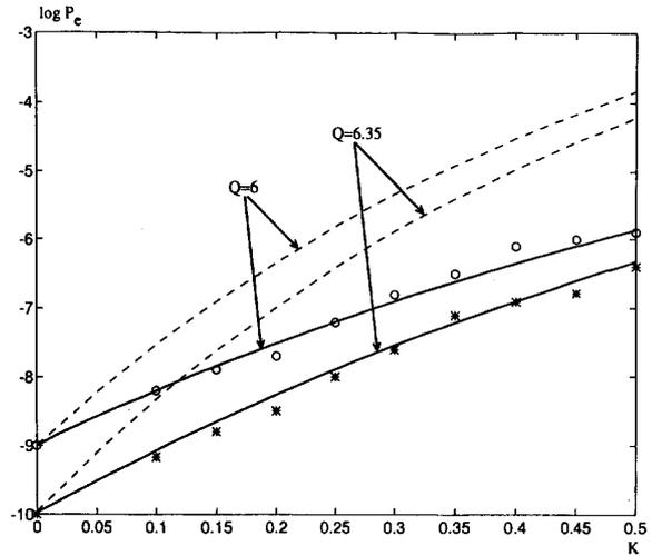
Fig. 3. BER performance of burst-mode receiver versus the decay parameter  $k$ . The dashed lines are the upper bounds computed from (4) and the solid lines are the result from the simulation experiment.
