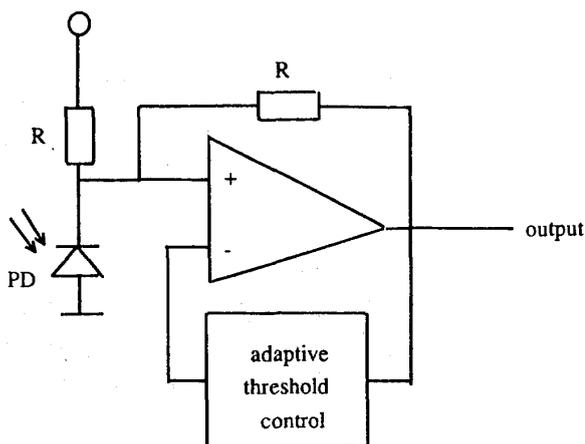
Fig. 1. Schematics of a burst-mode receiver.
