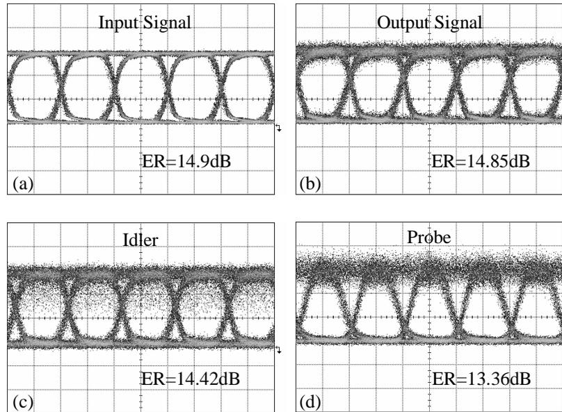
Fig. 2 Eye diagrams for (a) input signal; (b) output signal; (c) idler; (d) probe with the corresponding extinction ratios of (a) 14.9 dB; (b) 14.85 dB; (c) 14.42 dB; (d) 13.36 dB
