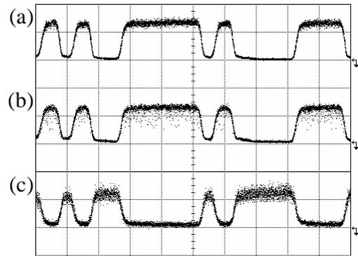
Fig. 4. Measured waveforms: (a) output signal; (b) idler; (c) probe.
