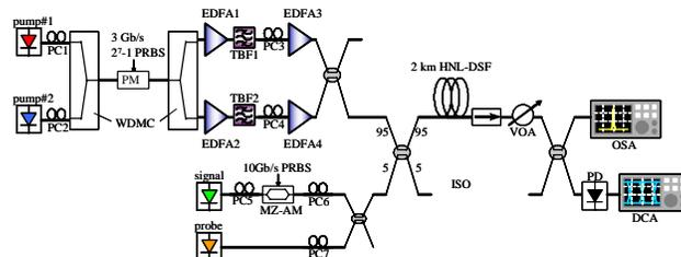
Fig. 1. 2-pump OPA configuration. TLS: Tunable laser source. PC: Polarization controller. PM: Phase modulator. VOA: variable optical attenuator. OSA: Optical spectrum analyzer. ISO: Isolator.
