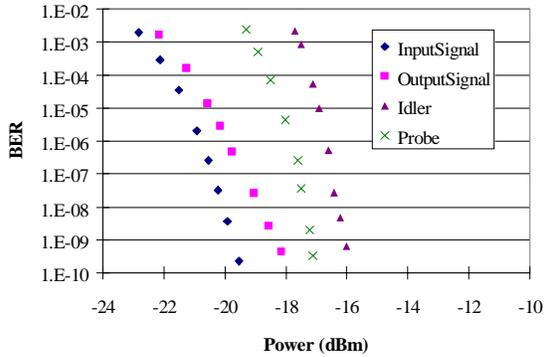
Fig. 3 Bit error rate of converted signals.
