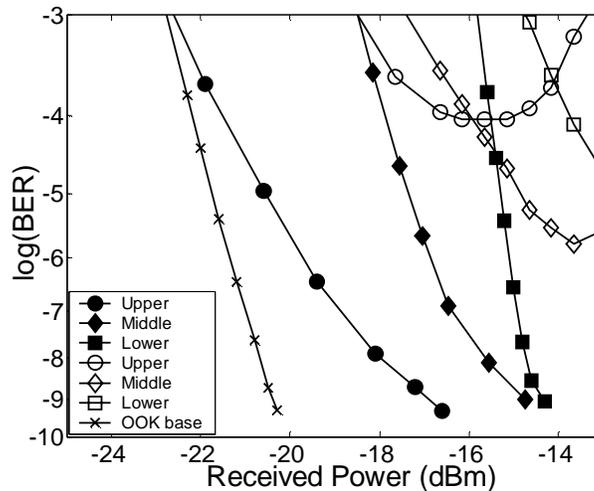
Fig. 4. BER curves for the upper eye (circle), the middle eye (diamond), and the lower eye (square) of the 4-ASK signal without (open) and with (solid) the all-optical decoding processing.
