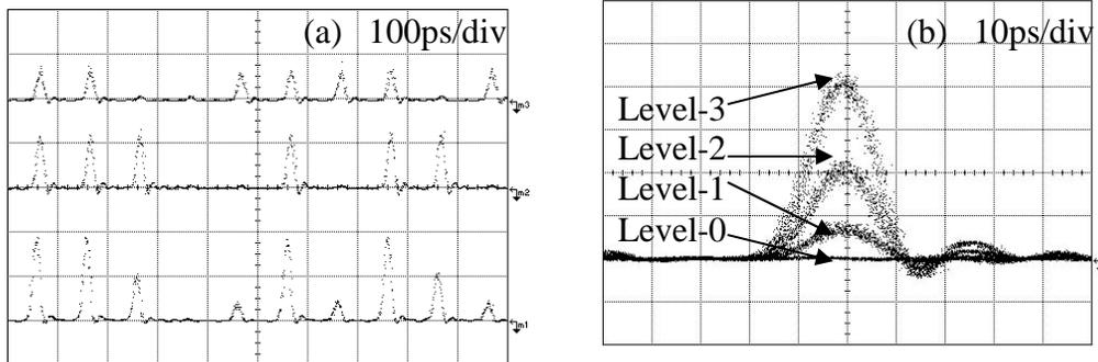
Fig. 2. The waveform (lower trace of (a)) and eye diagram (b) of 4-ask signal. XAM output signals when only 10dBm (upper trace) and 13dBm (middle trace) data was injected are also shown in (a).
