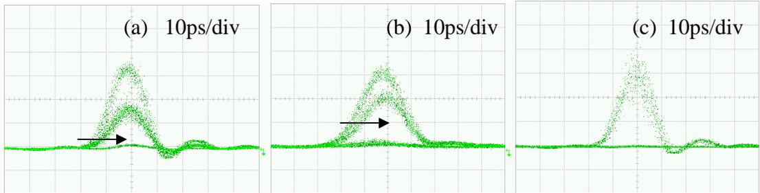
Fig. 3. Eye diagrams of the three separated 2-level eye patterns after the OBPF-2. (a), (b), and (c) correspond to the converted 2-level signals from the lower eye, the middle eye, and the upper eye of the 4-ASK signal, respectively. Arrows in (a) and (b) indicate the target eyes.
