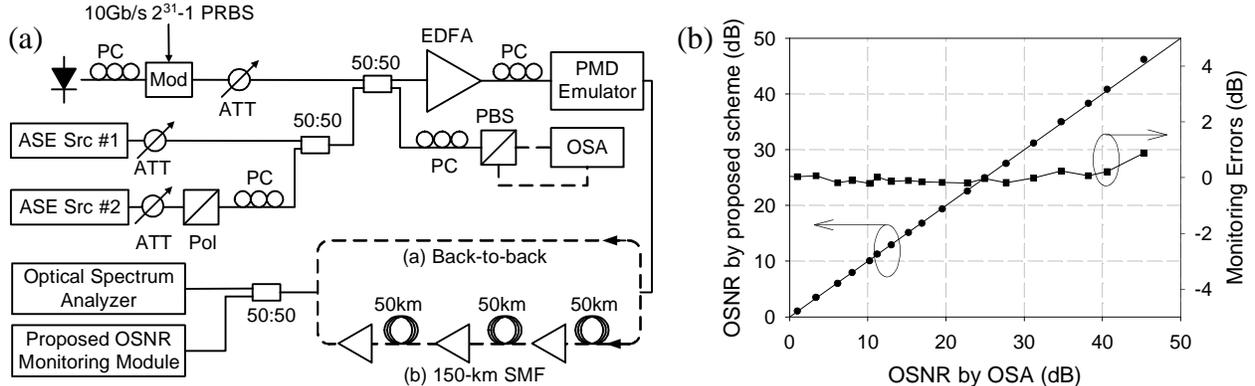
Fig. 2. (a) Experimental setup. PC: polarization controller, ATT: optical attenuator, OSA: optical spectrum analyzer, EDFA: erbium doped fiber amplifier; (b) Measured OSNR and monitoring errors
