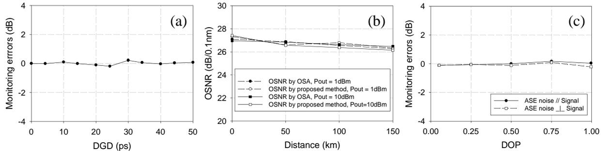
Fig. 3. (a) Monitoring errors under different DGDs for 25-dB OSNR; (b) OSNR monitoring results in a 150-km SMF link (PMD < 1.5ps, Pout=1 and 10 dBm respectively); (c) Monitoring errors for partially polarized ASE with different DOPs and alignment (dark for parallel, white for orthogonal) to signal for 25-dB OSNR
