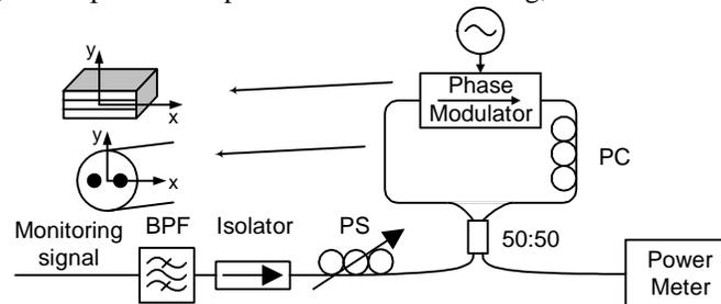
Fig. 1. Schematic diagram of the proposed OSNR monitoring module. PC: polarization controller, BPF: optical bandpass filter, PS: polarization scrambler.
