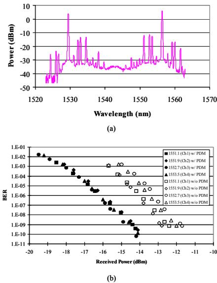
Fig. 2. (a) Spectrum of 2OP-OPA with three POIN signals; (b) BER curves for all four channels with and without POIN.
