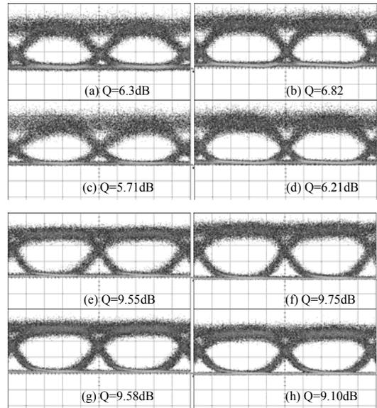
Fig. 3. Eye diagrams (with Q factors) for 2OP-OPA without POIN at different  $\lambda_s$  (nm): (a) 1551.1; (b) 1551.9; (c) 1552.7; (d) 1553.5. The corresponding eye diagrams with POIN (e) – (h).
