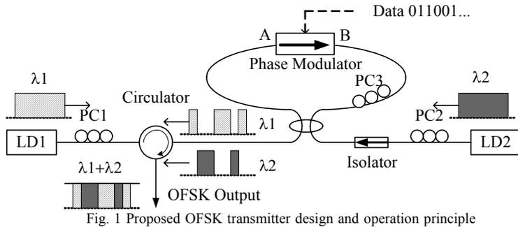
Fig. 1 Proposed OFSK transmitter design and operation principle
