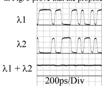
Fig.3 Measured waveforms of individual wavelengths and the composite signal
