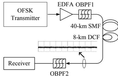
Fig.2 Experiment Setup. Inset shows the waveform of the OFSK signal after transmission
