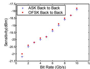
Fig.5 Receiver sensitivity of ASK and demodulated OFSK signals
