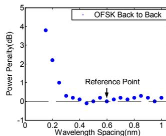
Fig.4 Power penalties for different wavelength spacing of demodulated OFSK signals
