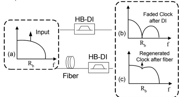
Fig. 1: Operation principle of the proposed dispersion monitoring scheme. RF spectrum of (a) input signal, signal after HB-DI (b) without and (c) with dispersion.
