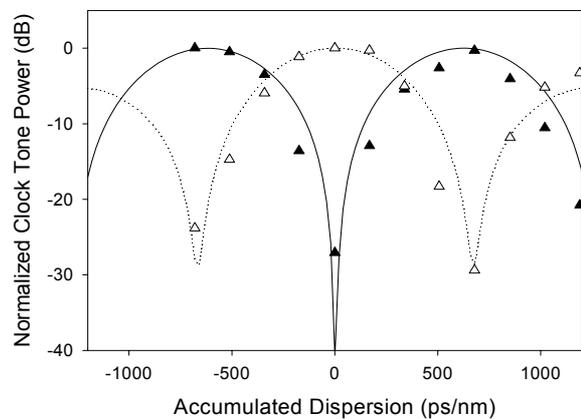
Fig. 3. Normalized RF power at 10 GHz as a function of accumulated dispersion for the previous (experiment: open symbol, simulation: dotted line) and proposed (experiment: filled symbol, simulation: solid line) schemes.
