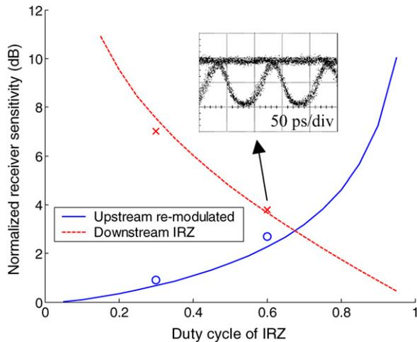
Fig. 4. The normalized back-to-back receiver sensitivities of the 10-Gb/s downstream IRZ and the 2.5-Gb/s upstream remodulated signals versus the IRZ duty cycle. Symbols indicate the experimental measurements while lines indicate the theoretical performance. The inset shows the measured eye diagram of the downstream IRZ signal.
