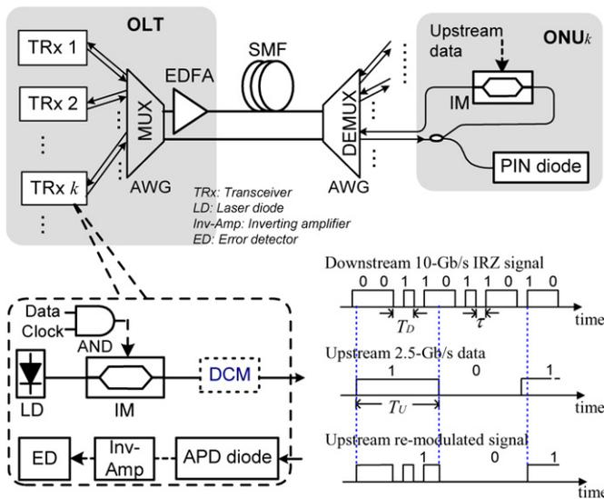
Fig. 1. The architecture schematic of the CLS WDM-PON employing downstream IRZ signals. The insets show typical waveforms of the downstream optical IRZ signal, the upstream data signal, and the remodulated upstream optical signal, respectively.
