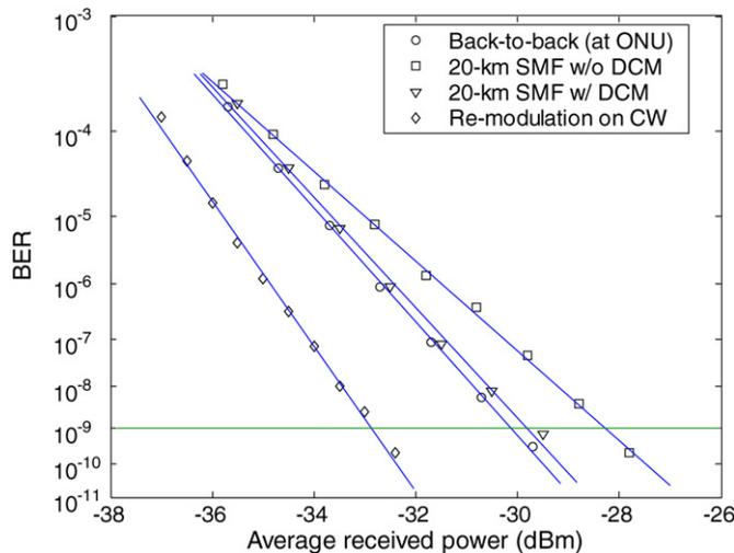
Fig. 3. BER measurements of the 2.5-Gb/s upstream remodulated signals.
