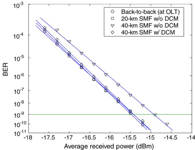
Fig. 2. BER measurements of the 10-Gb/s downstream IRZ signals.
