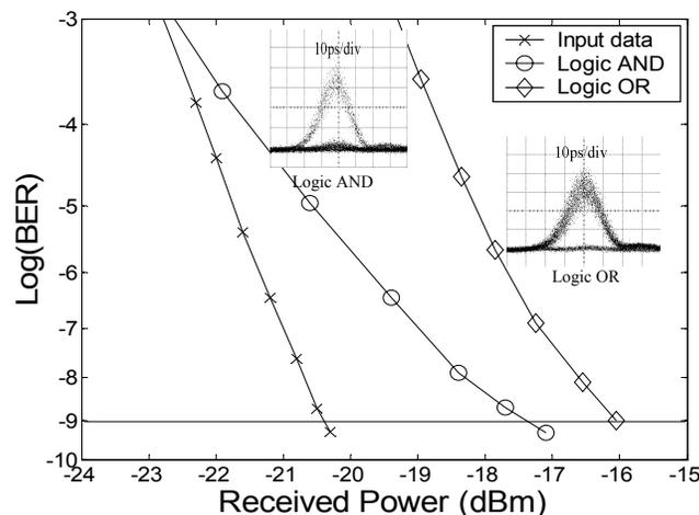
Fig. 4. BER curves for the input data (cross), the AND function (circle), and the OR function (diamond). The eye diagrams corresponding to the AND and OR functions are also presented as the insets, time scale: 10ps/div
