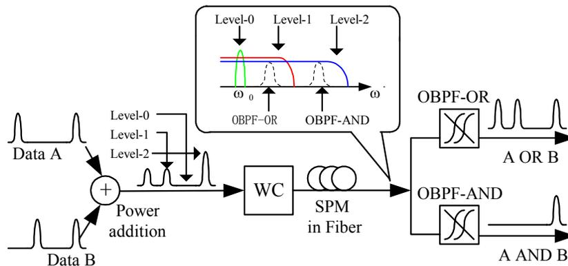
Fig. 1. Operation principle of the multilevel modulation based reconfigurable AND/OR logic gate
