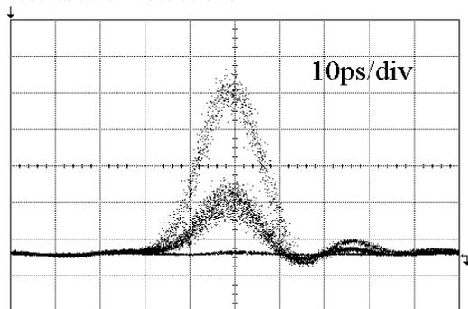
Fig. 3. Eye diagram of the wavelength converted three-level signal
