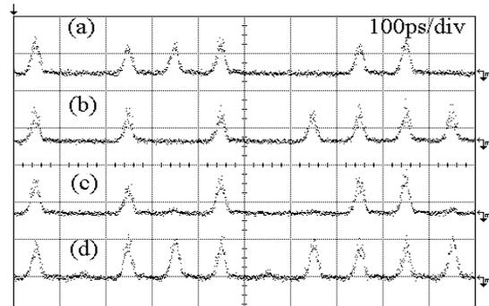
Fig. 4. Waveforms for the input data, and the resulting logic outputs (a) data A, (b) data B, (c) A AND B, (d) A OR B
