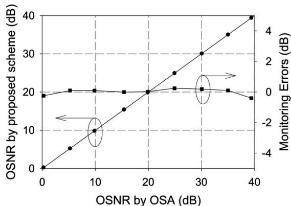
Fig. 7. Measured OSNR and monitoring errors for 2.5 Gbit/s data rate.
