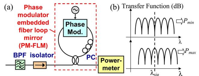
Fig. 1. (Color online) (a) Schematic diagram of a transmission link with the proposed OSNR monitoring module. PC, polarization controller; (b) Illustrated PM-FLM transfer function when destructive and constructive interference for the data signal occurs.
