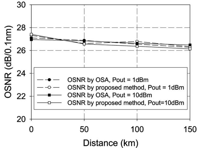
Fig. 4. OSNR monitoring results in a 150 km SMF link (PMD < 1.5 ps).
