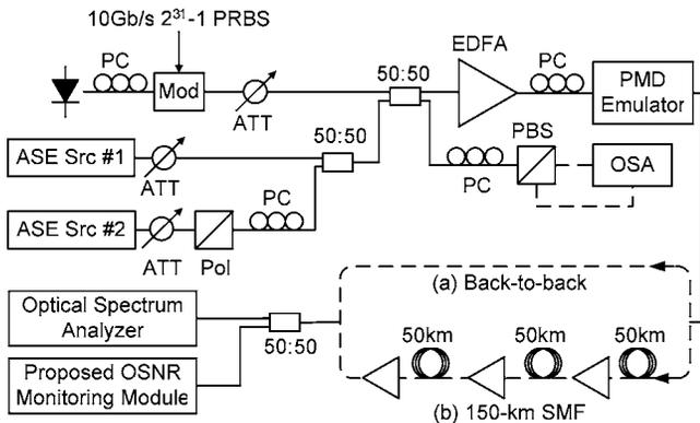
Fig. 2. Experimental setup. ATT; optical attenuator.
