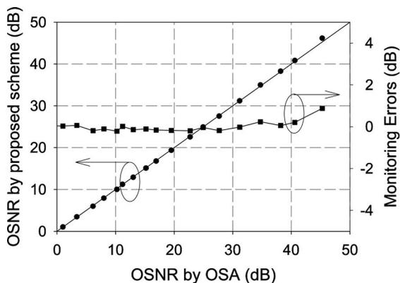
Fig. 3. Measured OSNR and monitoring errors.
