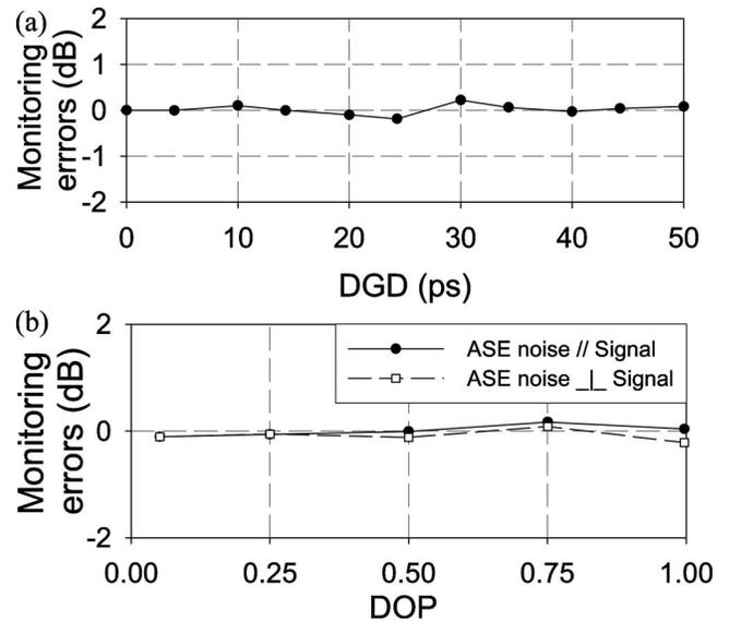
Fig. 5. Monitoring errors for (a) different DGDs and (b) partially polarized ASE with different DOPs and alignment to signal, for 25 dB OSNR.
