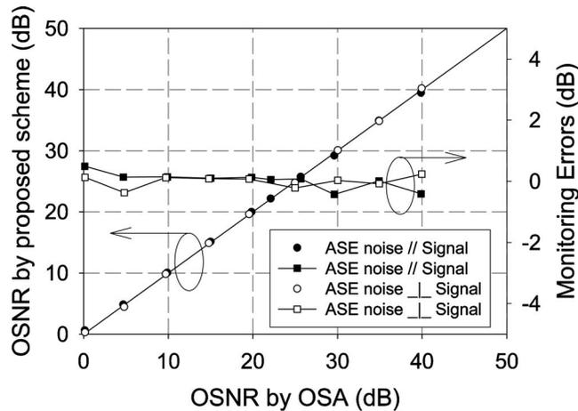
Fig. 6. Measured OSNR (circles) and monitoring errors (squares) for polarized ASE (DOP=99.69%) that is parallel (black) or orthogonal (white) to signal.
