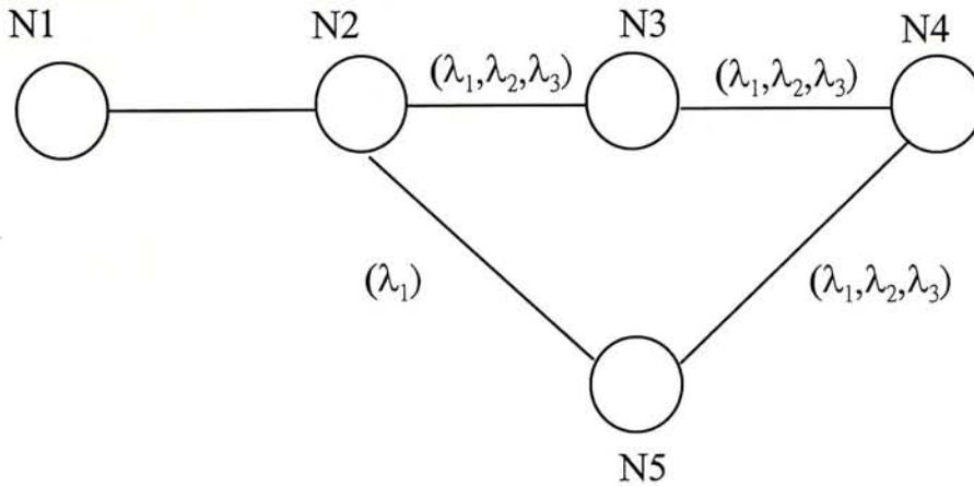
**Figure 7a** Initial wavelength assignments for our illustrative network.
