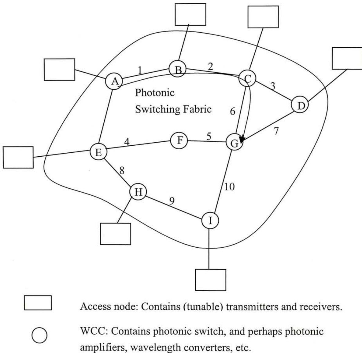
Fig. 1 A wavelength-routing (wide-area) optical network.
