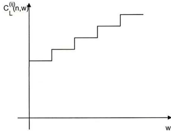
**Figure 8.** Typical fiber installation cost as a function of fiber number  $w$ .
