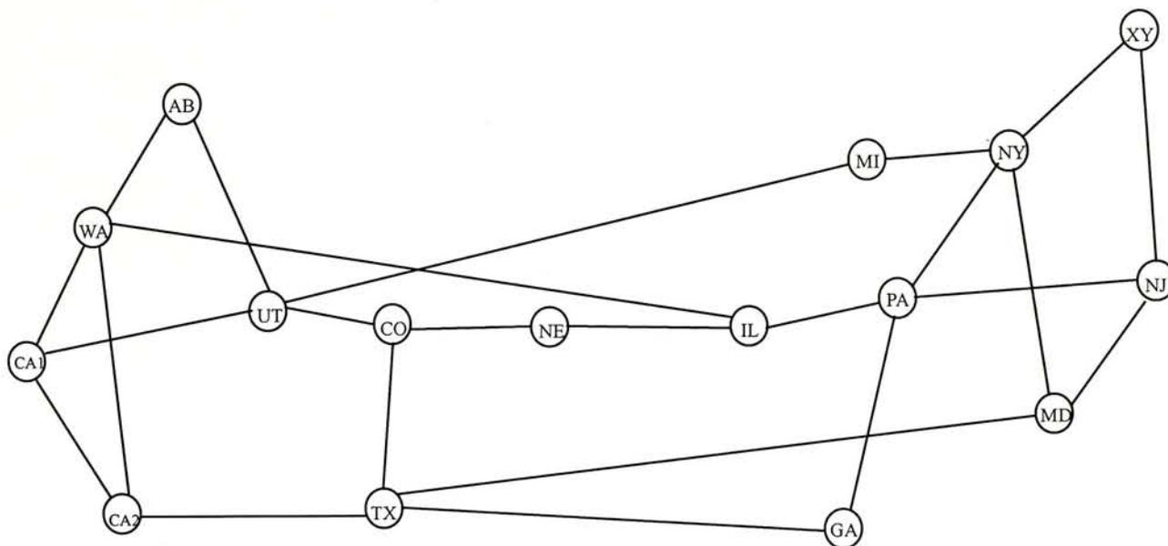
Fig.14. Physical topology of the NSFNET backbone network.
