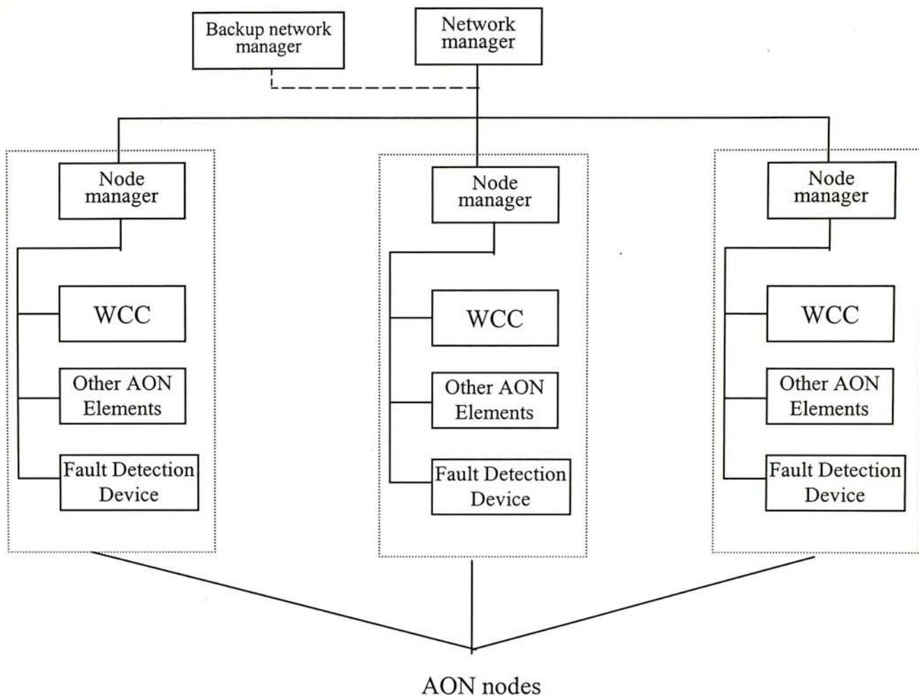
Figure 10. The relations between the different elements.
