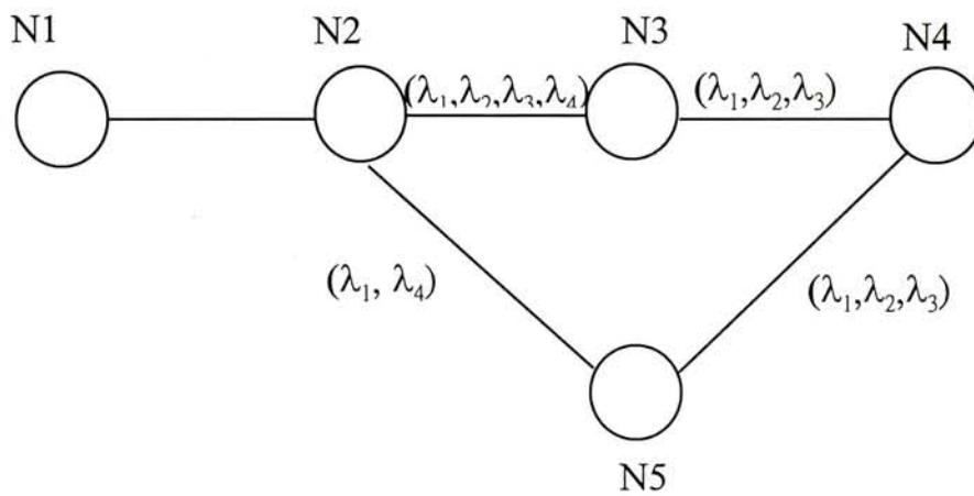
**Figure 7c.** Wavelength assignment after a lightpath is setup by using  $\lambda_4$  on the path  $r_{325}$  when SPA is used.
