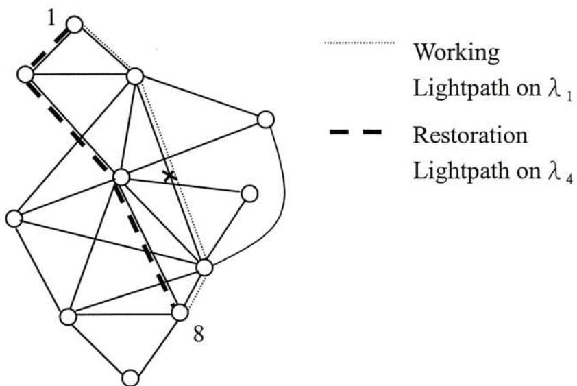
Figure 13. Source based restoration for the working lightpath between node 1 and node 8 by setting up a new lightpath not passing through the cut edge.
