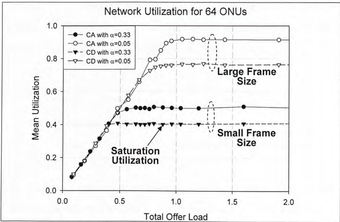
Figure 3.8 Effect of Loading on Utilization
