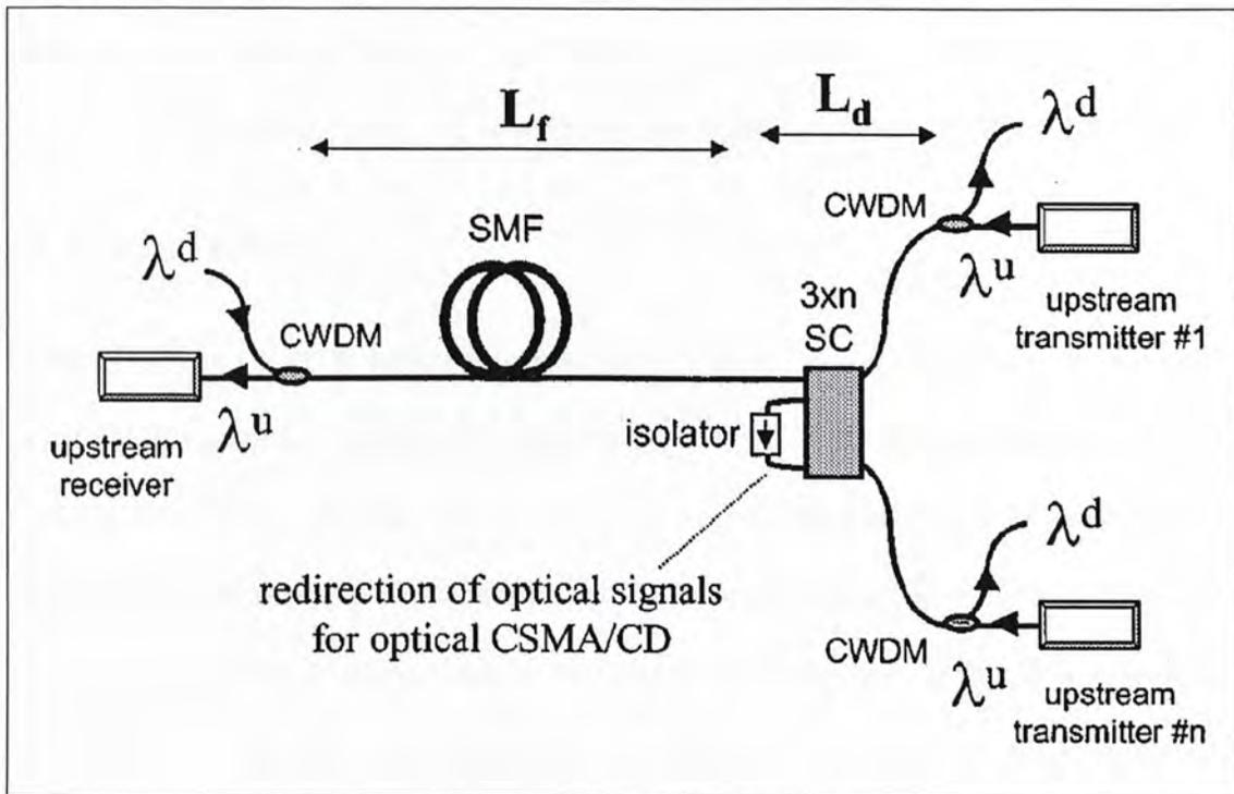
Figure 2.4 Schematic of CSMA/CD over EPON [13]
