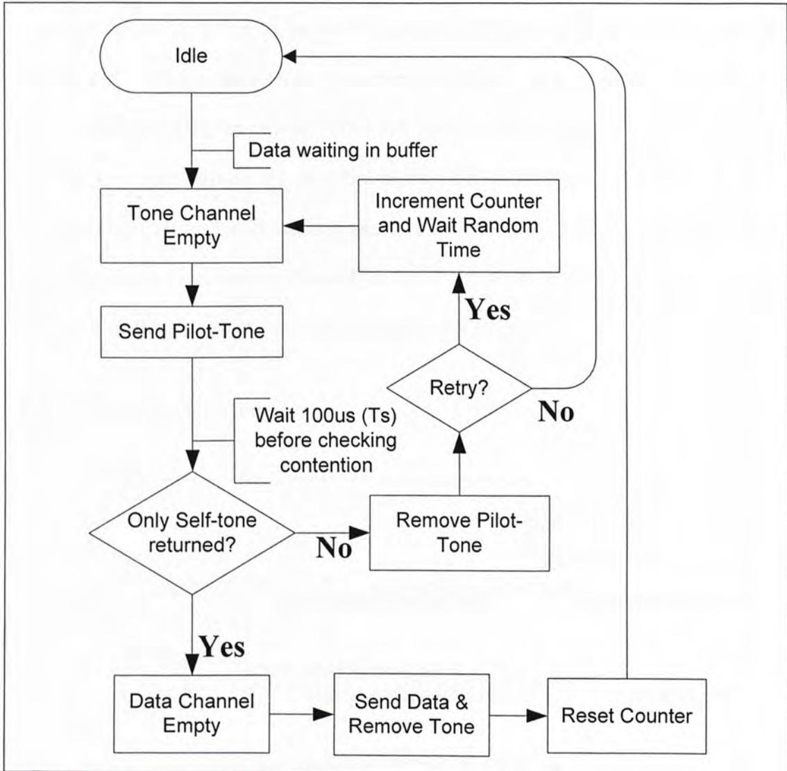
Figure 3.2 CSMA/CA protocol using Pilot Tone on PON
