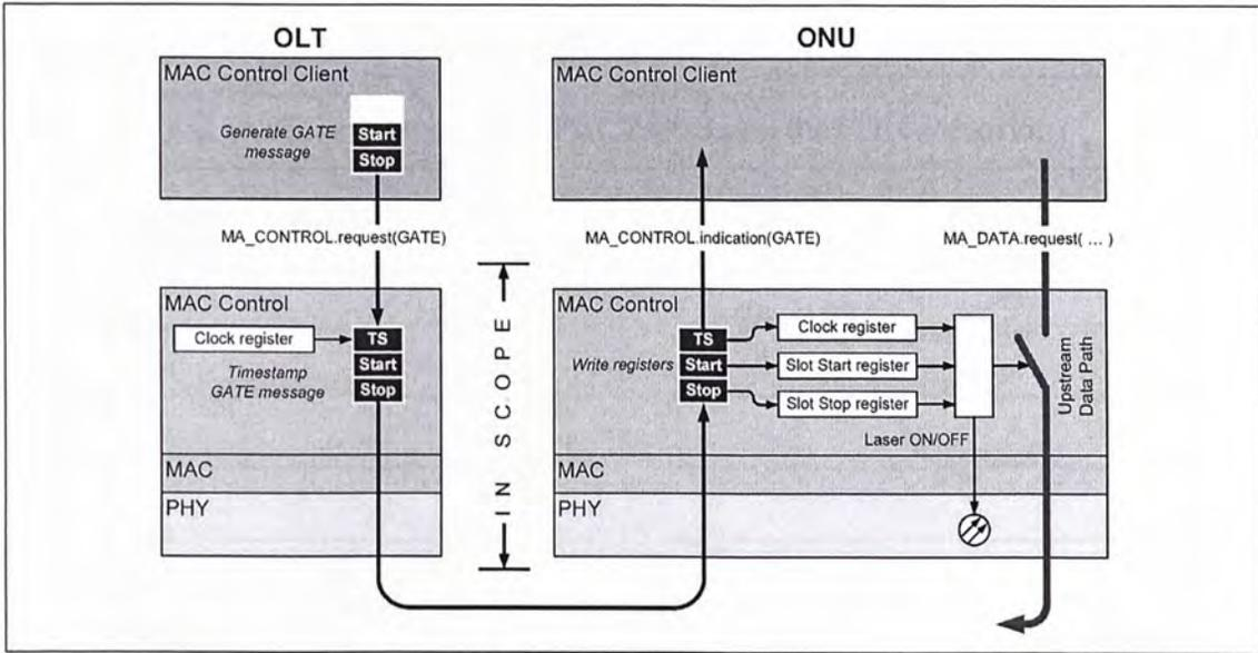
Figure 2.1 Sending GATE Message with MPCP [IEEE 802.3ah]
