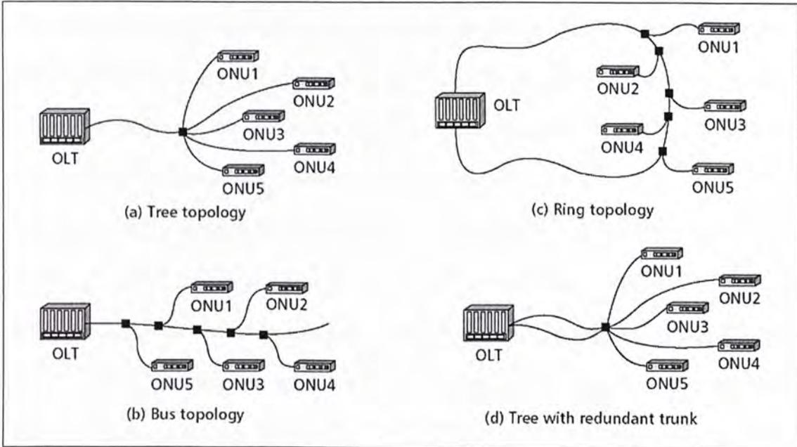
Figure 1.2 Typical PON Architecture
