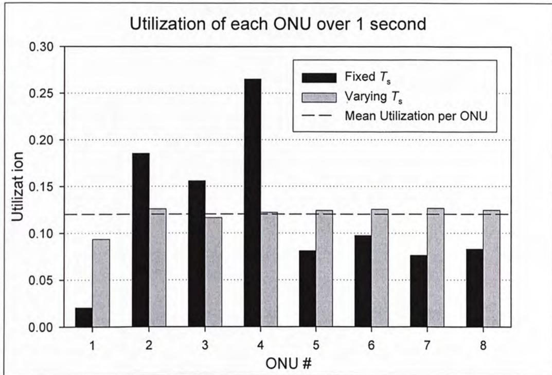
Fig. 4.5 Simulation on Utilization of 8 ONUs over 1 second
