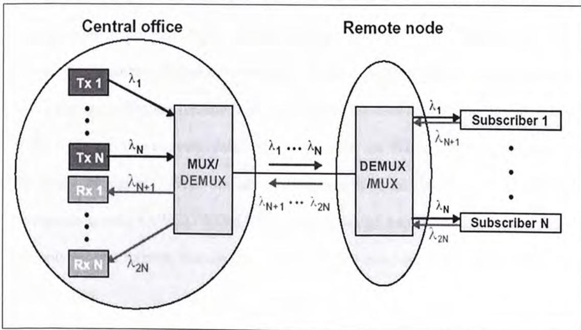
Figure 1.4 WDM PON Architecture
