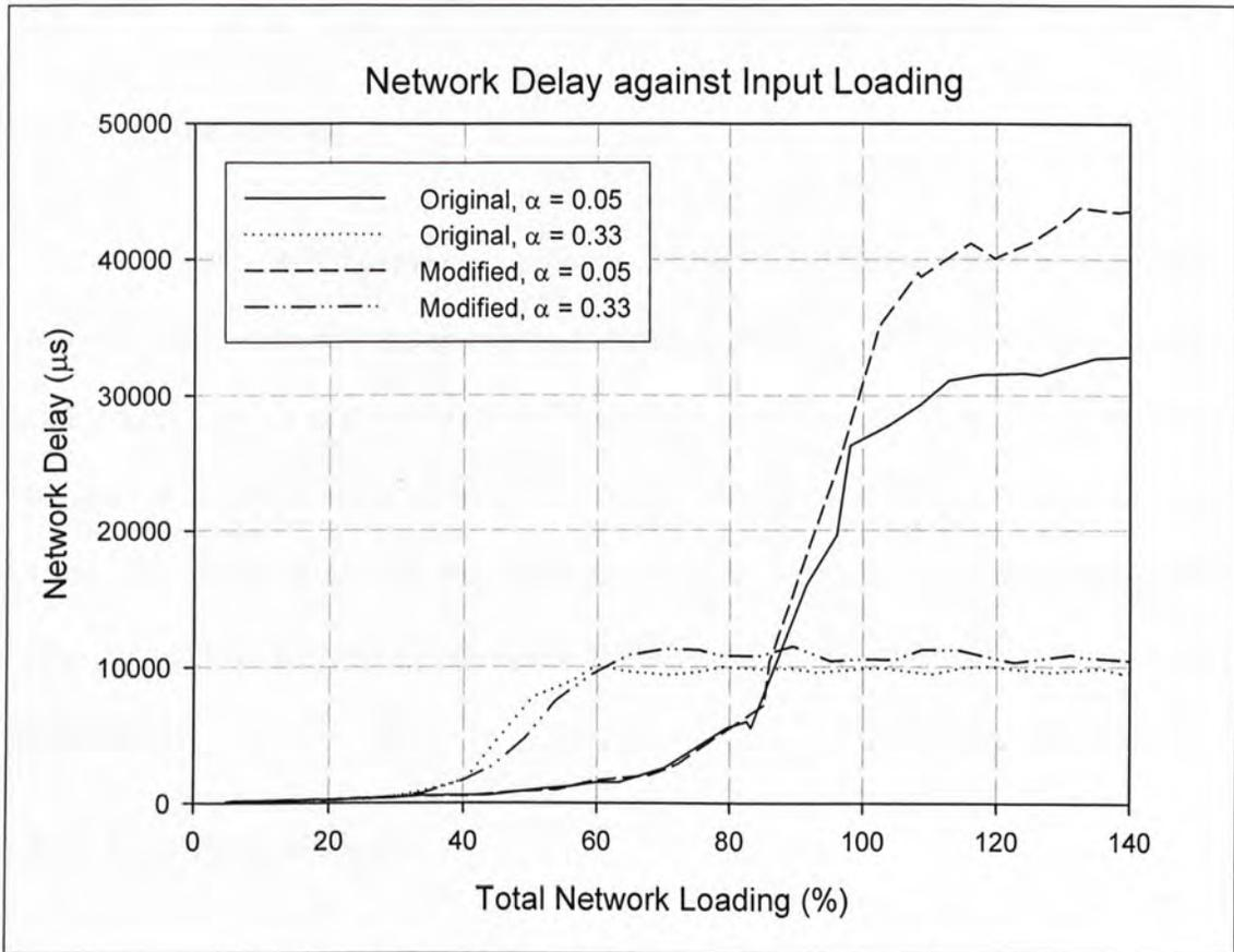
Figure 4.4 Network Delay against input loading
