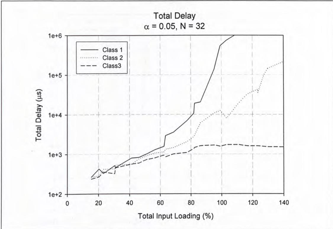
Figure 4.11 Total Delay for 3 different classes of service
