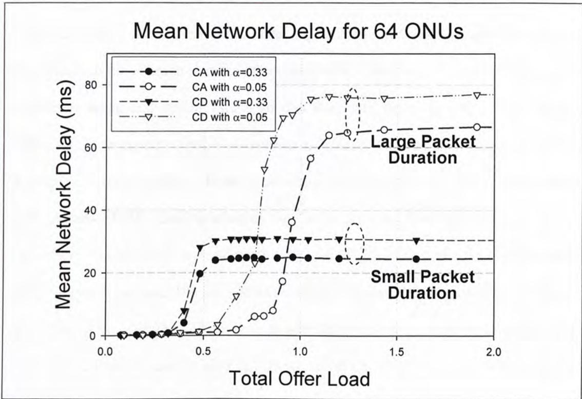
Figure 3.10 Effect of loading on delay
