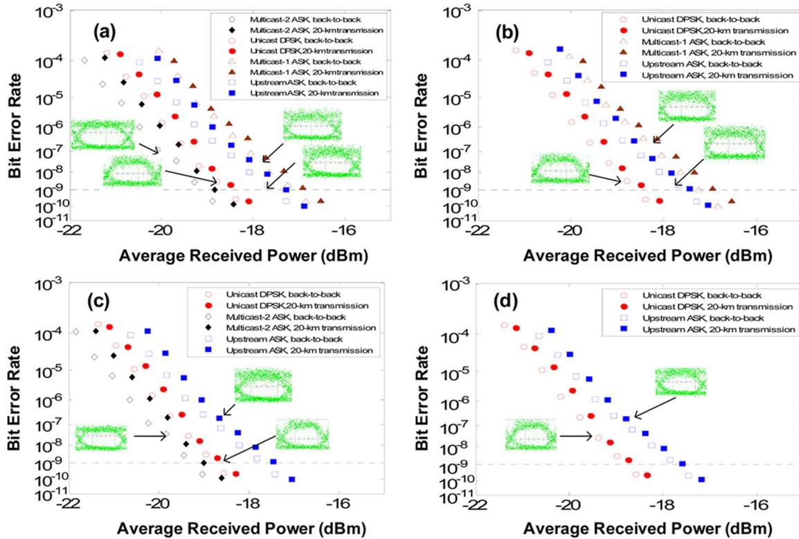
Fig. 4. BER measurements of 10-Gb/s transmissions. (a) Both multicast data streams are enabled; (b) only Multicast data 1 is enabled; (c) only Multicast data 2 is enabled; (d) both multicast data streams are disabled. Time scale for eye diagrams: 50 ps/div.
