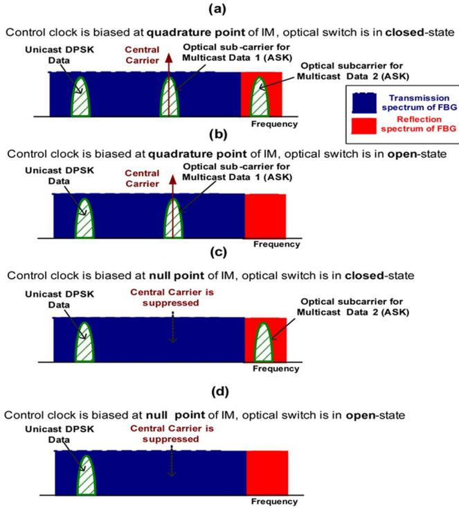
Fig. 2. Spectra of downstream carrier to illustrate the principle of multicast overlay fiber control via control clock and optical switch. (a) Both Multicast data 1 and Multicast data 2 enabled. (b) Only Multicast data 1 enabled. (c) Only Multicast data 2 enabled. (d) Both Multicast data 1 and Multicast data 2 disabled.
