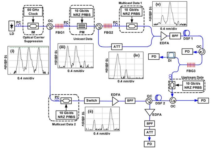
Fig. 3. Experimental setup. Insets show the (i) output spectrum of the IM; (ii) reflected spectrum of FBG1 (i.e., Multicast data 2); (iii) transmitted spectrum of FBG1; (iv) spectrum for unicast data; (v) spectrum for Multicast data 1. OC: optical circulator; BPF: bandpass filter; ATT: optical attenuator.
