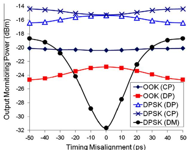
Fig. 4. Experimental results of output monitoring power for different timing misalignments using 94-ps DI.
