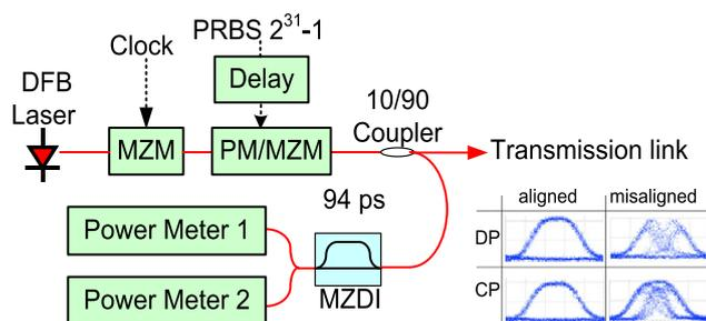
Fig. 3. Experimental setup. Inset: Eye diagrams of the detected RZ-DPSK signals from each port of the DI when the pulse carver and data modulator are well aligned or have half-bit misalignment. Time scale: 20 ps/div. DP: destructive port and CP: constructive port.
