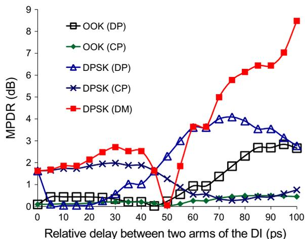
**Fig. 6.** MPDR versus the delay of DI when the RZ-DPSK/RZ-OOK signals are generated by single-modulator. DP: destructive port, CP: constructive port, and DM: differential monitoring.
