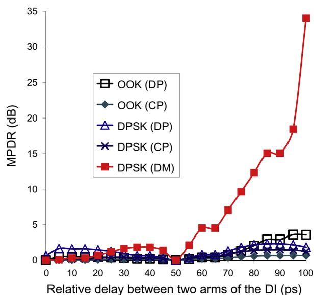
Fig. 5. MPDR vs. the delay of DI. The duty cycle of the RZ pulse train in simulation was 33%. DP: destructive port, CP: constructive port, and DM: differential monitoring.
