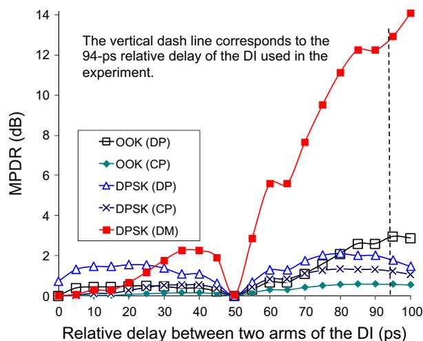
Fig. 2. MPDR versus the delay of DI. The duty cycle of the RZ pulse train in simulation was 50%. DP: destructive port, CP: constructive port, and DM: differential monitoring.
