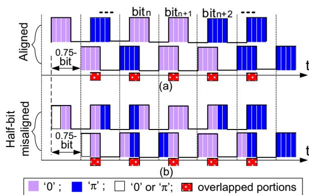
Fig. 1. RZ-DPSK signals in the two arms of the DI before combining by the output 3-dB coupler for (a) aligned and (b) half-bit misaligned cases.
