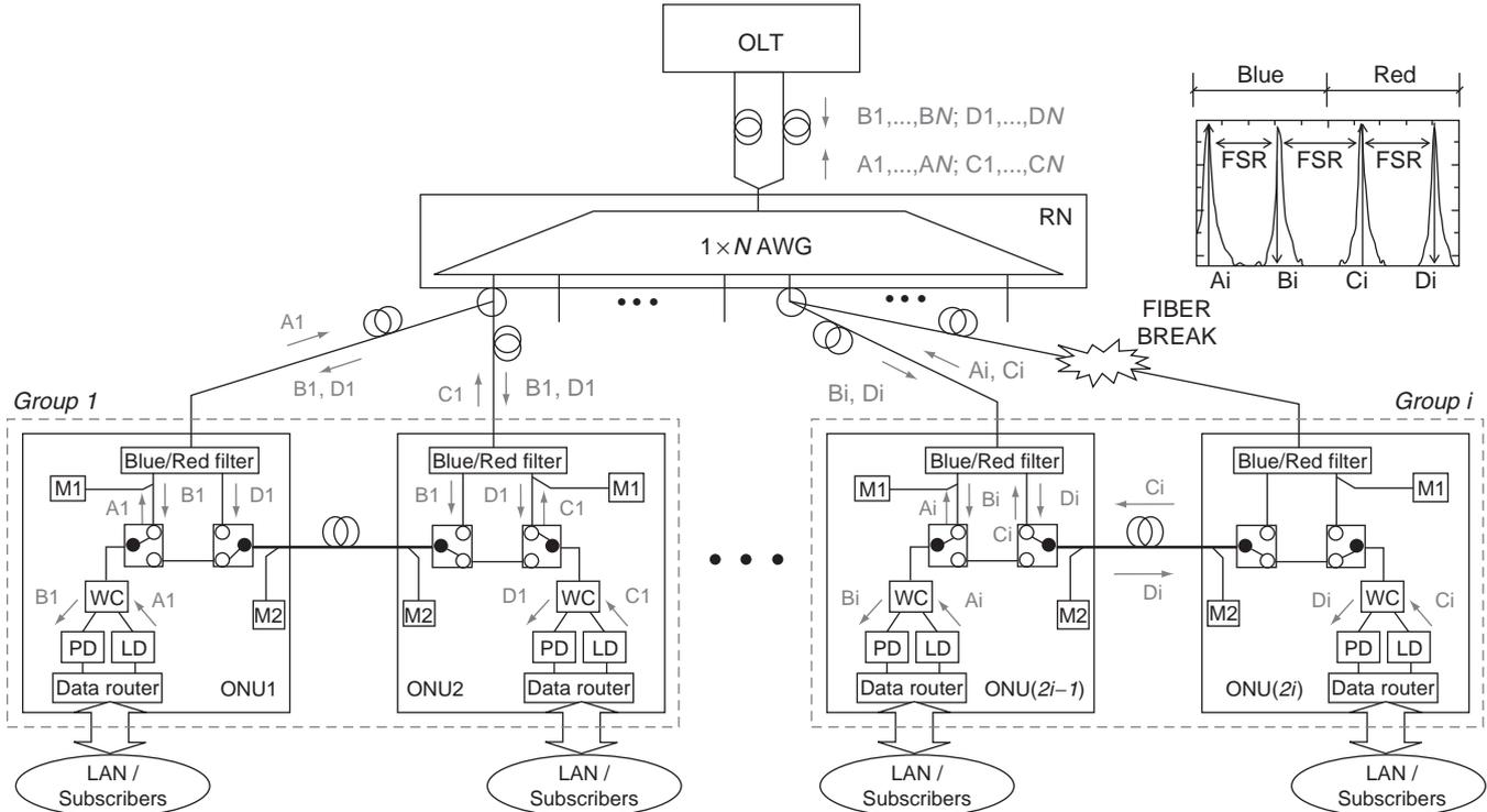
**Figure 6.9** Self-protected network architecture for WDM-PON. LD1–4: laser diode; PD1–4: PIN photodiode; WC: WDM coupler; M1&M2: optical power monitors;  $\{A_i, C_i\}$  for  $i \in \{1, \dots, N\}$ : upstream wavelengths;  $\{B_i, D_i\}$  for  $i \in \{1, \dots, N\}$ : downstream wavelengths. Inset shows the spectral response of one of the output ports of the AWG. FSR: free-spectral range of the AWG [28].
