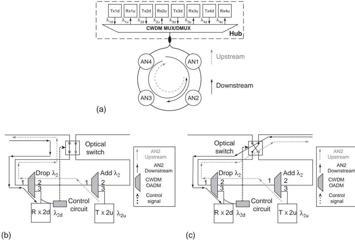
**Figure 6.12** (a) A single-fiber CWDM optical access ring network; (b) & (c) the structure of AN2 in (b) normal state and (c) protection state when there was a fiber cut between AN2 and AN3 [45]. AN: access node, Tx: transmitter, Rx: receiver.
