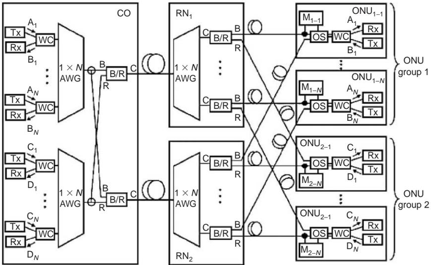
**Figure 6.11** A WDM-PON architecture with self-protection capability against both feeder fiber and distribution fiber failures [32]. WC: wavelength coupler, B/R: blue/red filter, OS: optical switch, M: power monitoring modules.
