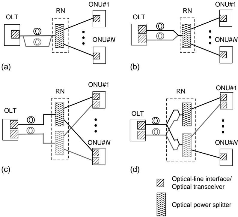
Figure 6.1 Protection switching architectures suggested by ITU-T G.983.1.
