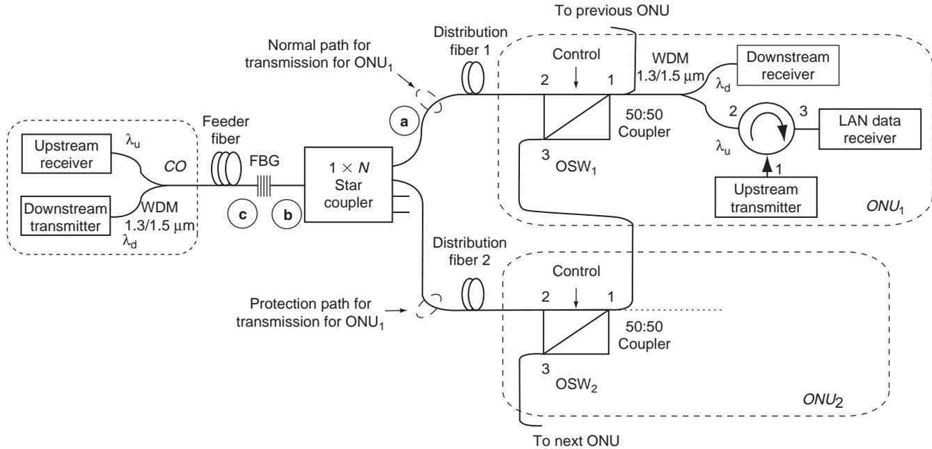
**Figure 6.3** A PON architecture with protection of distribution fibers by interconnecting ONUs with protection switching [17]. OSW: optical switch, FBG: fiber Bragg gratings,  $\lambda_d$ : downstream wavelength,  $\lambda_u$ : upstream wavelength.
