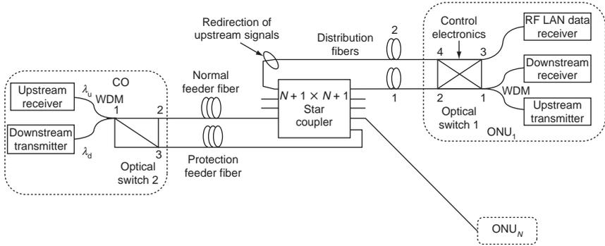
**Figure 6.4** A PON architecture with protection of both feeder and distribution fibers by an additional loopback distribution fiber with protection switching [18].  $\lambda_d$ : downstream wavelength,  $\lambda_u$ : upstream wavelength.
