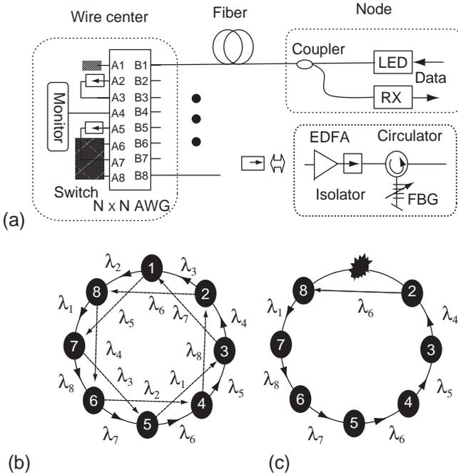
**Figure 6.13** (a) A protected optical star-shaped ring network; (b) lightpath diagram, dotted lines were the designated protection paths; (c) the protection lightpath was adopted when node 1 failed [47]. FBG: fiber Bragg gratings.
