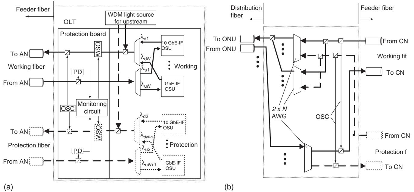
**Figure 6.8** The structure of (a) the OLT and (b) RN of a WDM-PON with duplicated fiber feeders for protection [27]. AN: access node, CN: central node, OSC: optical supervisory channel, PD: photodiode, OSW: optical switch.
