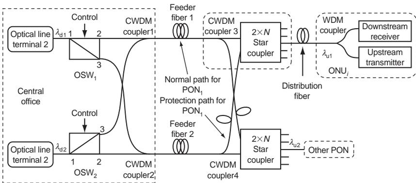
**Figure 6.5** Protection of feeder fibers in two PONs using CWDM technology [19]. OSW: optical switch,  $\lambda_d$ : downstream wavelength,  $\lambda_u$ : upstream wavelength.
