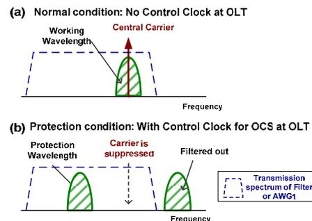
Fig. 2: Spectra of downstream carrier to illustrate the principle.
