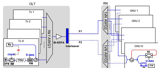
Fig. 1: Proposed survivable WDM-PON architecture.
