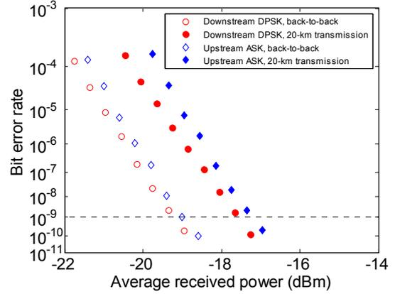
Fig. 4: BER measurements in the working (normal) mode.
