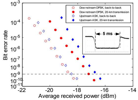
Fig. 5: BER measurements in the protection mode.
