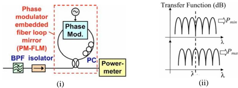
Fig. 2 (i) A schematic diagram of a proposed OSNR monitoring module using polarization modulator embedded fiber loop mirror (PM-FLM). PC, polarization controller; (ii) Illustrated PM-FLM transfer function when destructive and constructive interference for the data signal occurs.
