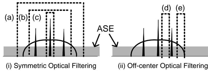
Fig. 1 Illustration of optical filtering scheme for DOP-based OSNR monitoring using symmetric or off-center optical filtering.
