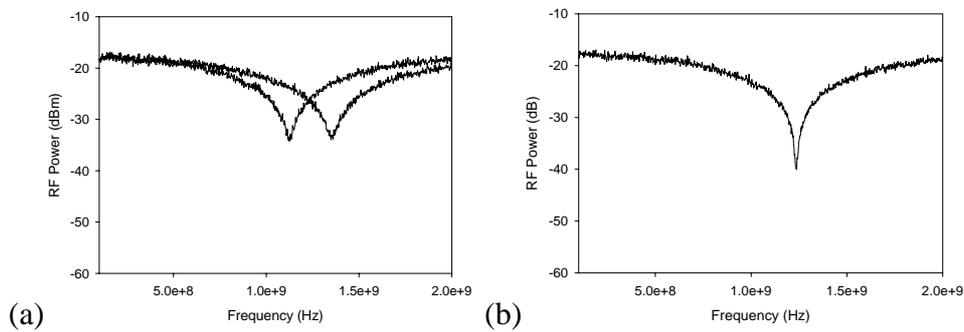
Fig. 5 (a) RF spectrum with the power dip shift with the large-DGD element of  $\sim 409$ ps and PMD emulator of 40ps, (b) RF spectrum with the minimum power measured at large-DGD element of  $\sim 409$ ps, PMD emulator of 20ps and OSNR of 35dB.
