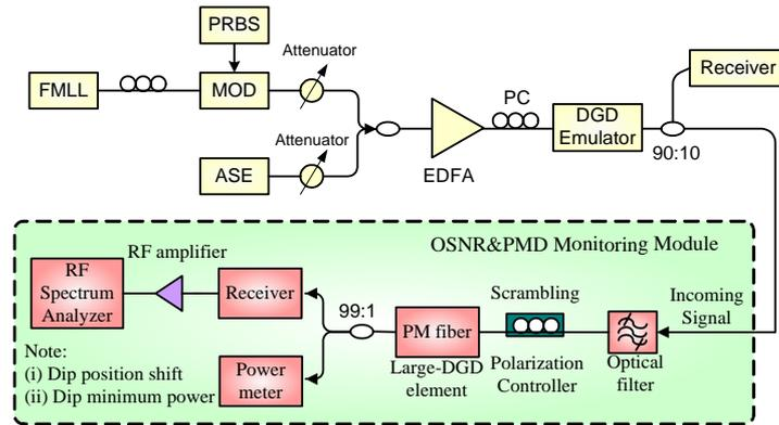
Fig. 4. Experimental setup for the PMD and OSNR simultaneous monitoring based on RF spectral dip monitoring
