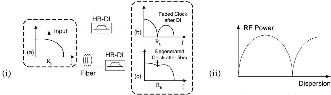
Fig. 3. (i) Operation principle of the proposed dispersion monitoring scheme. RF spectrum of (a) input signal, signal after HB-DI (b) without and (c) with dispersion; (ii) RF power of clock tone as function of dispersion in the proposed scheme.
