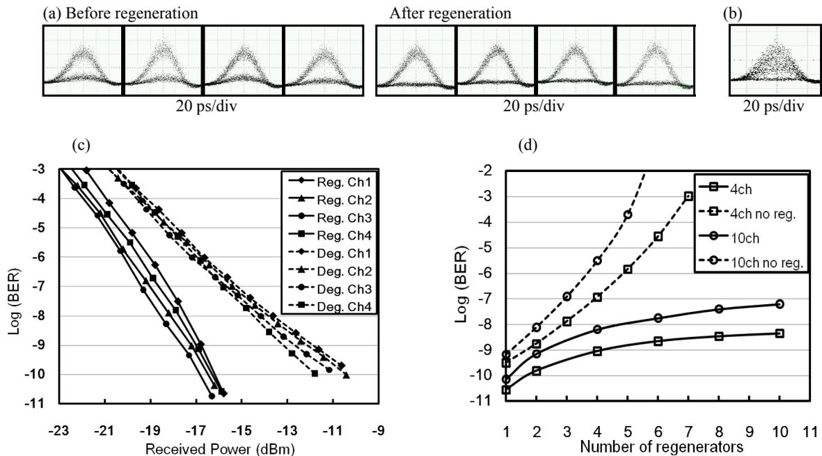
Figure 3. (a) Eye diagrams of the 4 channels before and after the regeneration, (b) Eye diagram of one regenerated WDM channel without proper inter-channel timing walk-off, (c) BER measurements of 4 channels before and after the regeneration, (d) BER evolution versus the number of inline regenerators for 4- and 10-channel operations in numerical simulation.
