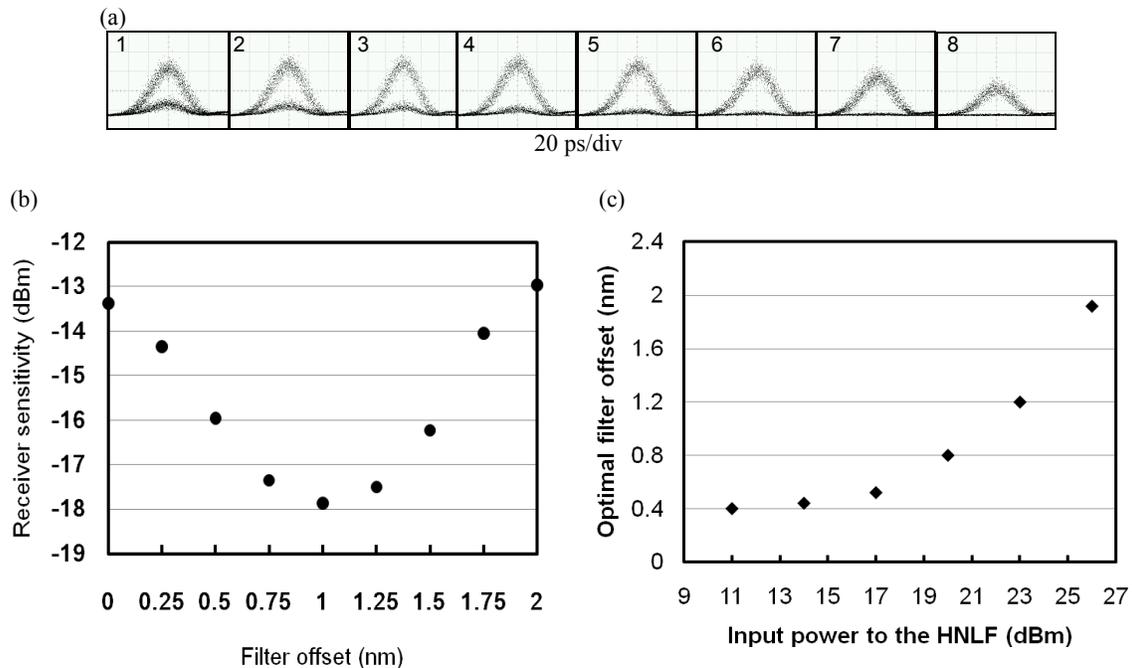
Figure 5. (a) 1-8, Eye diagrams of one regenerated signal as the filter offset is increased with a 0.25-nm step. (b) Receiver sensitivity of one WDM channel at BER of  $10^{-9}$  versus different filter offsets in the experiment. (c) Optimal filter offset versus signal power launched into the HNLF in numerical simulations.
