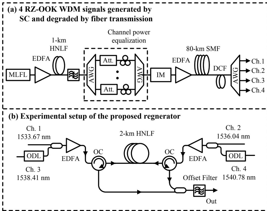
Figure 2. Experimental setup. MLFL: mode-locked fiber laser; IM: intensity modulator; Att.: attenuator; ODL: optical delay line. AWG: arrayed waveguide grating.
