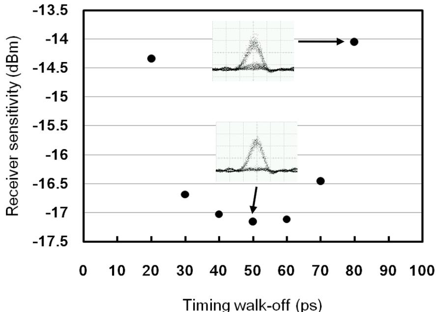
Figure 4. Receiver sensitivity of channel 1 (1533.67 nm) at BER of  $10^{-9}$  versus different timing walk-off values of channel 3 (1538.41 nm) in the same propagation direction in regeneration.
