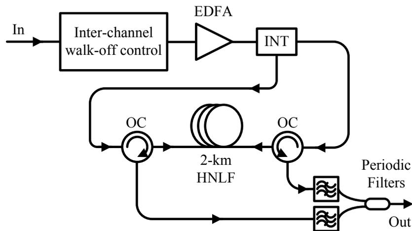
Figure 1. Proposed system architecture of the multi-wavelength 2R regenerator based on SPM and inter-channel walk-off control. EDFA: erbium-doped fiber amplifier; HNLF: highly nonlinear fiber; INT: interleaver; OC: optical circulator.
