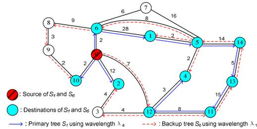
Fig. 2: An example of the established multicast primary tree  $S_1$  (solid arrowed lines) and its respective backup tree  $S_6$  (dashed arrowed lines).
