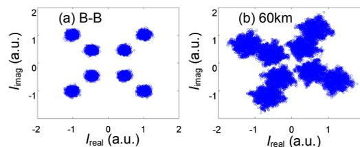
Fig. 2. Constellation of 8-ASK-QPSK signal at 6.84dB ER
