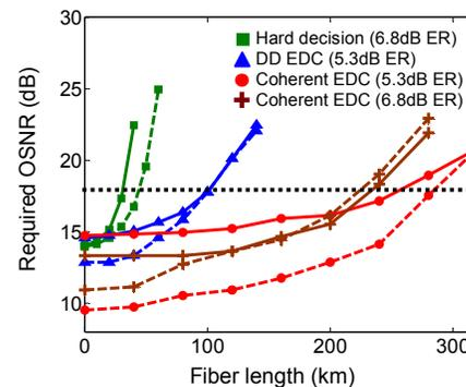
Fig. 4. Required OSNR versus fiber length for the ASK (solid) and DQPSK (or QPSK) (dashed) tributaries.
