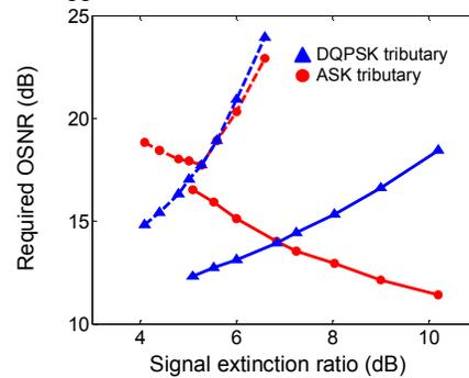
Fig. 3. Required OSNR versus ER for 8-ASK-DQPSK signal using hard decision at back-to-back (solid), and using DD EDC at 100km (dashed).
