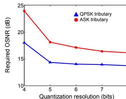
Fig. 5. Required OSNR versus quantization resolution for coherent detection based EDC at 5.3dB ER and 240km
