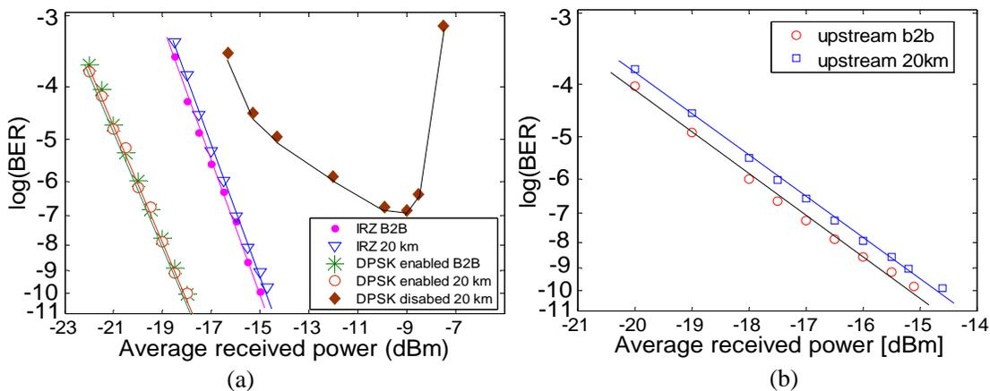
Fig. 3. BER curves: (a) downstream point-to-point signals and multicast signals ; (b) upstream signals.
