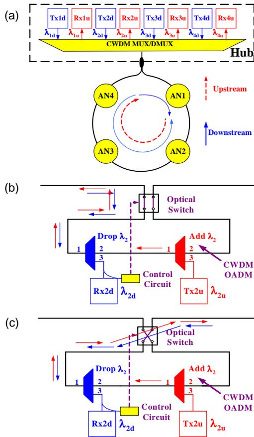
Figure 3: (a) A single-fiber CWDM optical access ring network; (b)&(c) the structure of access node AN2 in (b) normal state; (c) protection state when there was a fiber cut between AN2 and AN3 [21].
