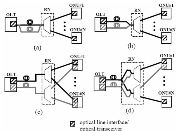
Figure 1: Protection switching architectures for WDM-PONs using the similar approaches suggested by ITU-T G.983.1.
