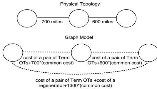
Fig.1. A graph model construction example based on physical topology when optical reach is 1200 miles
