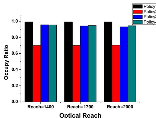
Fig. 2. Normalized network cost of four policies with different optical reaches
