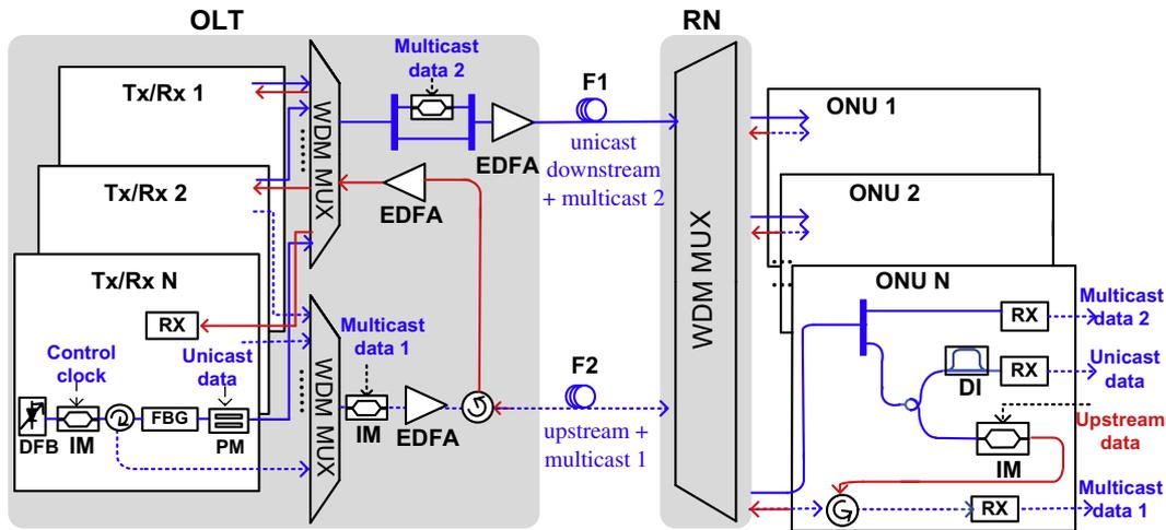
Fig. 1. A WDM-PON with proposed multicast overlay scheme. DFB: distributed feedback laser; EDFA: erbium-doped fiber amplifier; PM: phase modulator.
