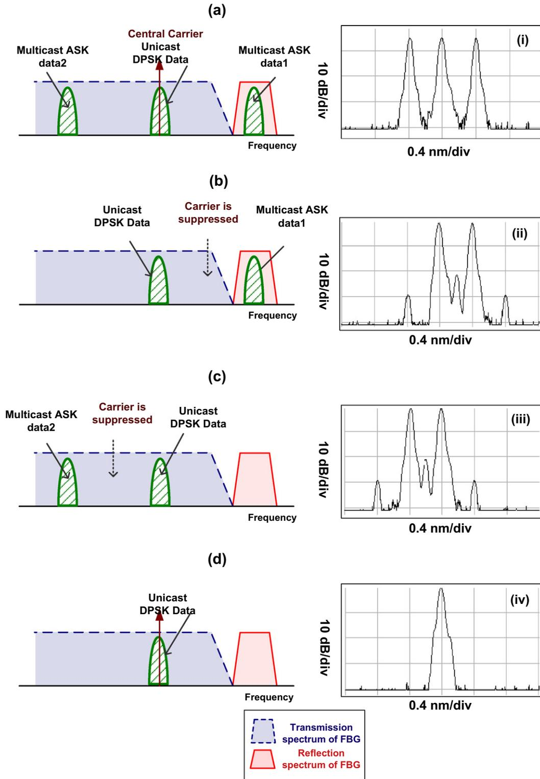
**Fig. 2.** Principle of multicast overlay fiber control. (a) Two Multicast Enabled: With Control Clock  $f$  and no wavelength shift. (b) One Multicast Enabled: With Control Clock  $f/2$  for OCS and wavelength right-shift  $f/2$ . (c) One Multicast Enabled: With Control Clock  $f/2$  for OCS and wavelength left-shift  $f/2$ . (d) Multicast Disabled: With no Control Clock and no wavelength shift.
