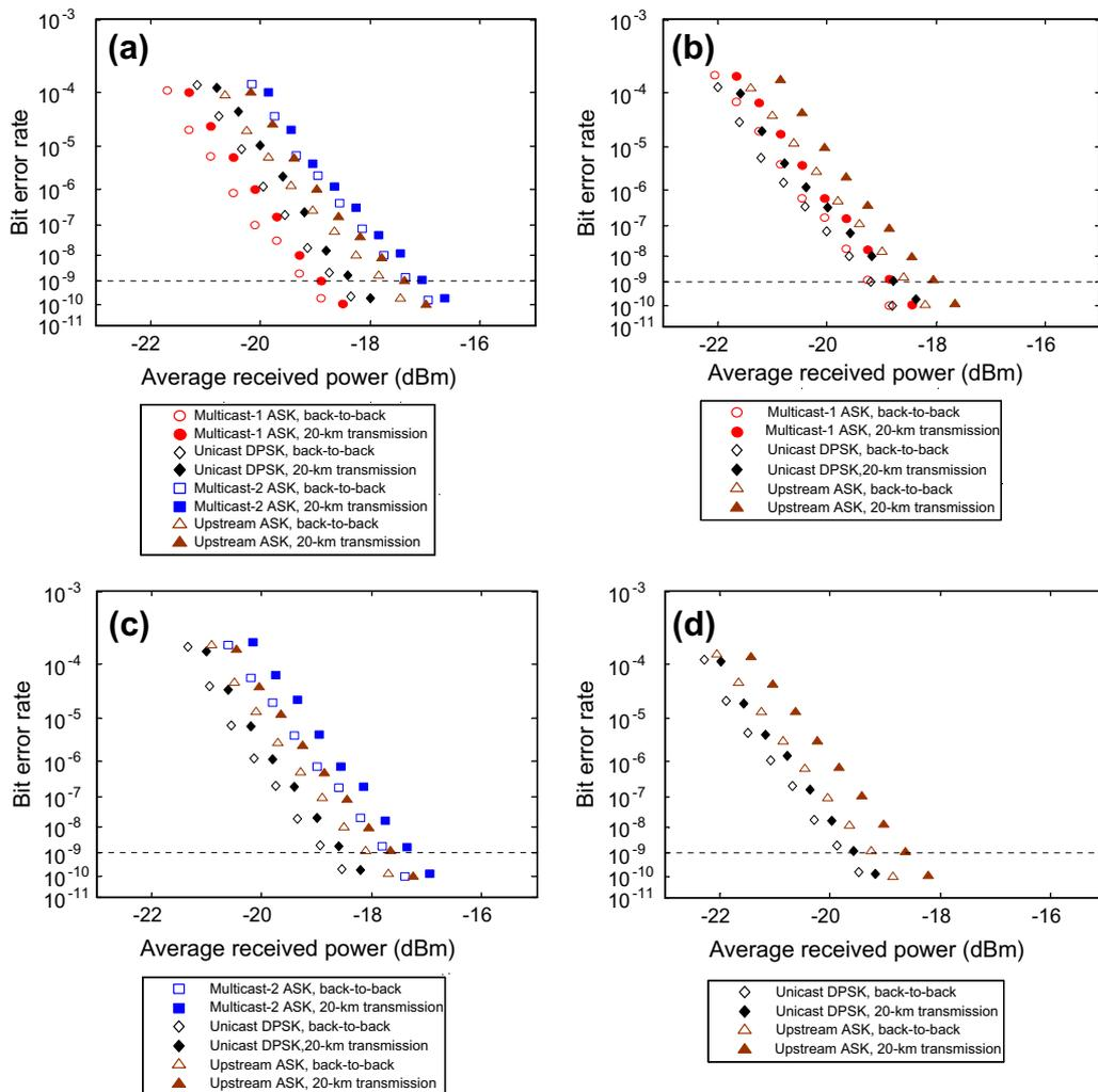
Fig. 4. BER measurements of 10-Gb/s transmissions: (a) both two multicast data streams are enabled; (b) only multicast data 1 is enabled; (c) only multicast data 2 is enabled; (d) both multicast data streams are disabled.
