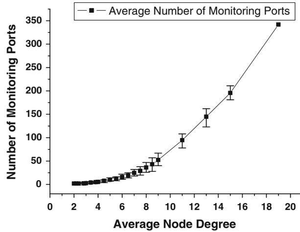
Fig. 12 Monitor cost (number of monitoring ports) versus AND with node number 20
