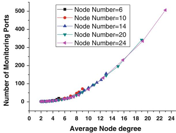
Fig. 14 Monitor cost (number of monitoring ports) versus AND with same node number
