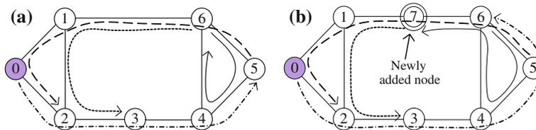
**Fig. 16** Monitoring solutions updated using different monitoring schemes (proposed scheme and M-Trail) when network topology changes (**a**) the original network (**b**) the new network (*shaded nodes* denote monitoring locations using proposed scheme and *arrows* denote monitoring trails using M-Trail scheme)
