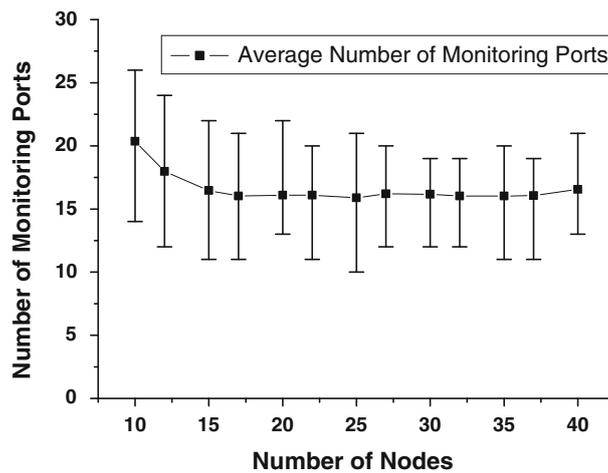
Fig. 7 Monitor cost (number of monitoring ports) versus node number with average node degree 6
