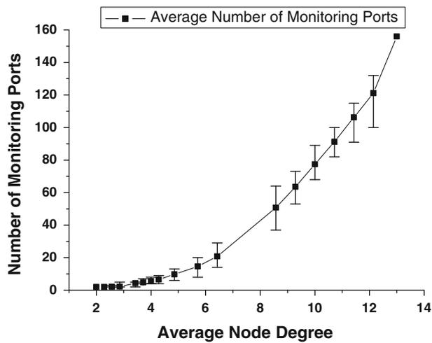
Fig. 11 Monitor cost (number of monitoring ports) versus *AND* with node number 14
