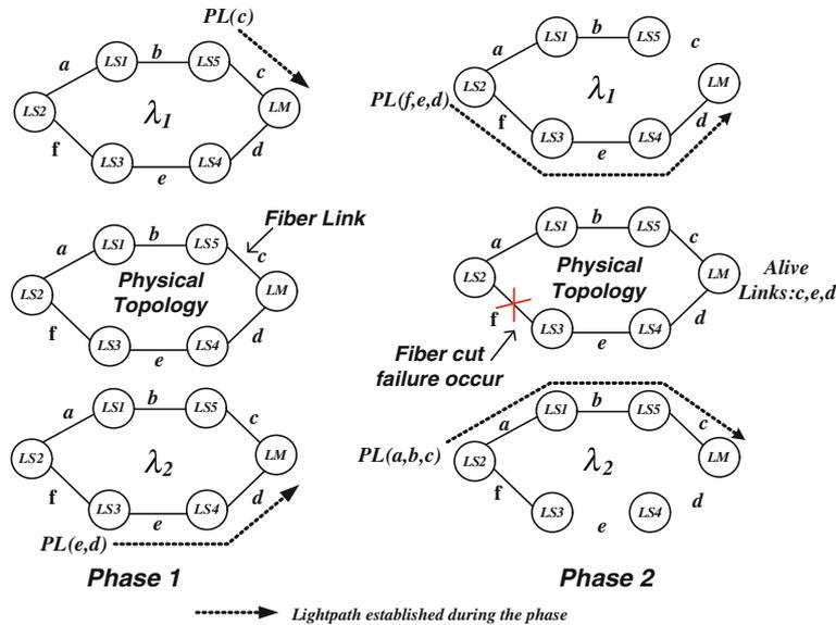
Fig. 4 An example to illustrate the procedures of Phase 2
