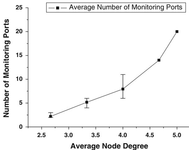
Fig. 9 Monitor cost (number of monitoring ports) versus *AND* with node number 6
