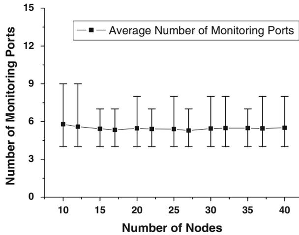
Fig. 6 Monitor cost (number of monitoring ports) versus node number with average node degree 4
