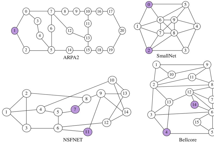
**Fig. 15** Several commonly used topologies for monitor number comparison (*shaded nodes* denote monitoring locations using proposed scheme)
