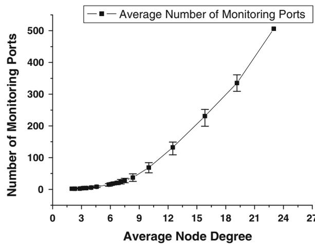
Fig. 13 Monitor cost (number of monitoring ports) versus AND with node number 24
