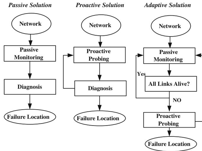
**Fig. 1** Fault monitoring solutions: passive, proactive, and adaptive
