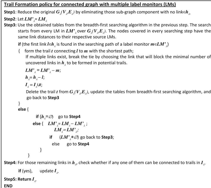
**Fig. 3** Flowchart of the algorithm to form monitoring trail set in each wavelength plane
