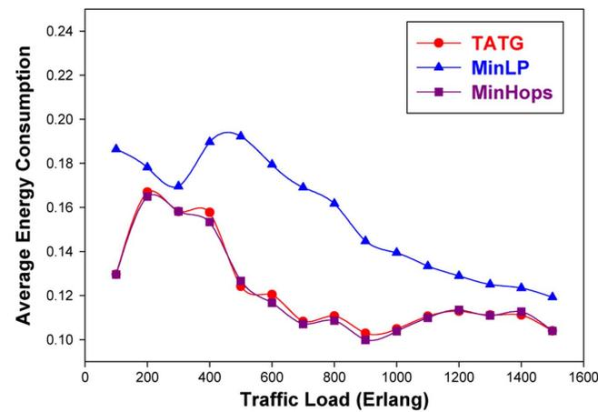
Fig. 12. Pacific Bell Net: average energy consumption per connection  $P_0 = 0$ .
