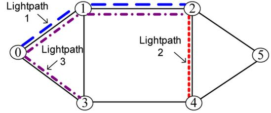
Fig. 1. Established lightpaths in the illustrative numerical example.
