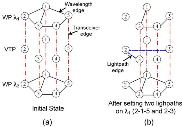
Fig. 2. (a) and (b) Example of a grooming graph. WP: wavelength plane, VTP: virtual topology plane, black solid line: wavelength edge, red dotted line (—•—): transceiver edge, blue dotted line (—•—): lightpath edge.
