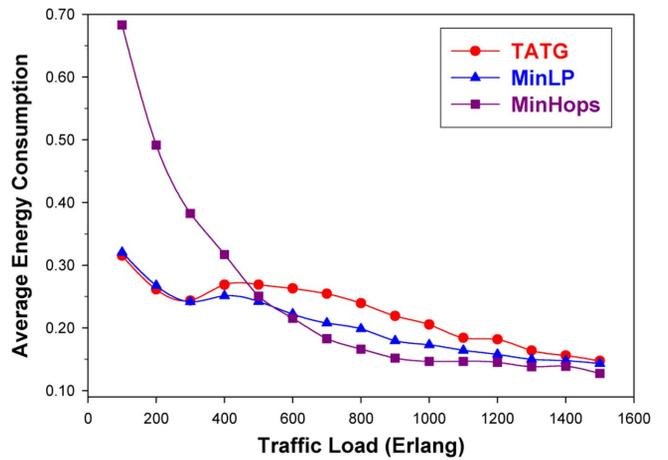
Fig. 14. Pacific Bell Net: average energy consumption per connection  $P_0 = 1$ .
