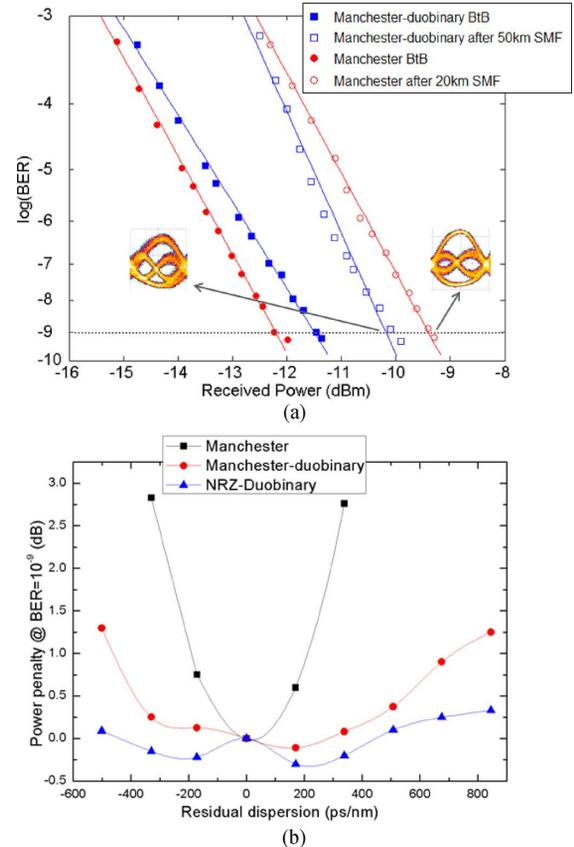
Fig. 3. Measured (a) BER performance, and (b) chromatic dispersion tolerance for 10-Gb/s Manchester-duobinary signal and conventional Manchester signal.
