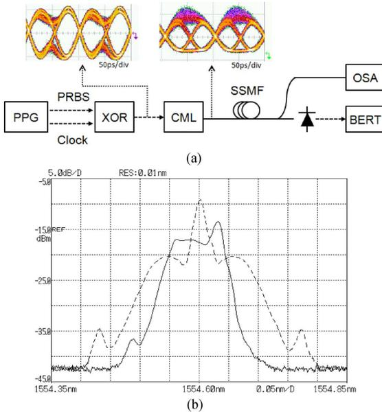
Fig. 2. (a) Experimental setup. (b) Optical spectra of 10-Gb/s conventional Manchester (dashed line) and Manchester-duobinary (solid line) signals.
