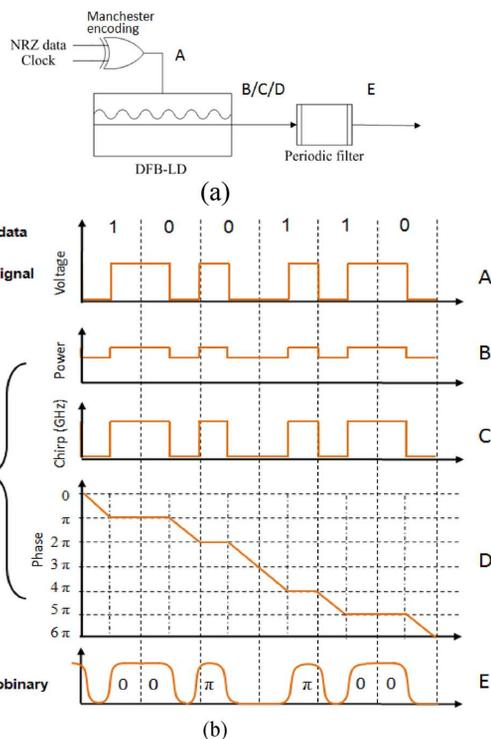
Fig. 1. (a) Schematic of CML-based Manchester-duobinary transmitter. (b) Illustration of the generation of the Manchester-duobinary signal.
