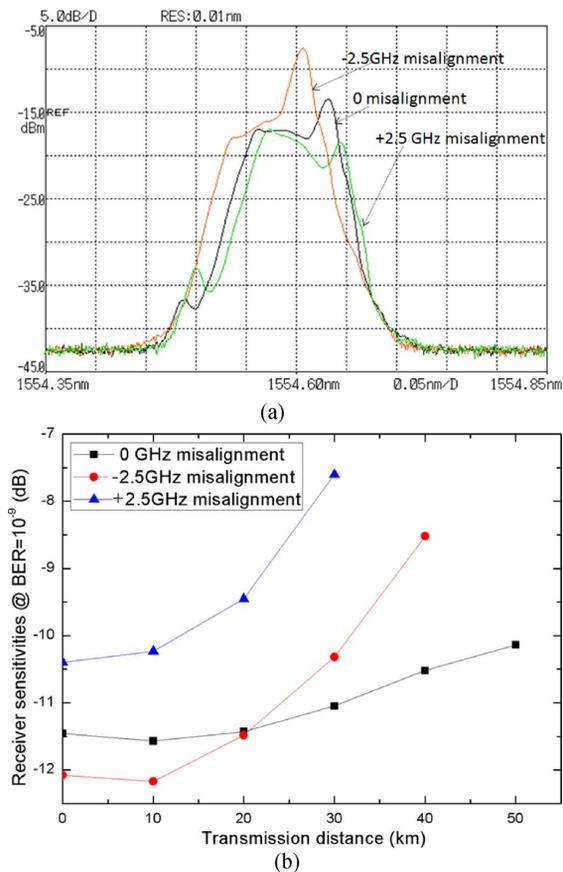
Fig. 4. (a) Optical spectra of the output Manchester-duobinary signal under different OSR operating points. (b) Receiver sensitivities as a function of transmission distance for different OSR operating points.
