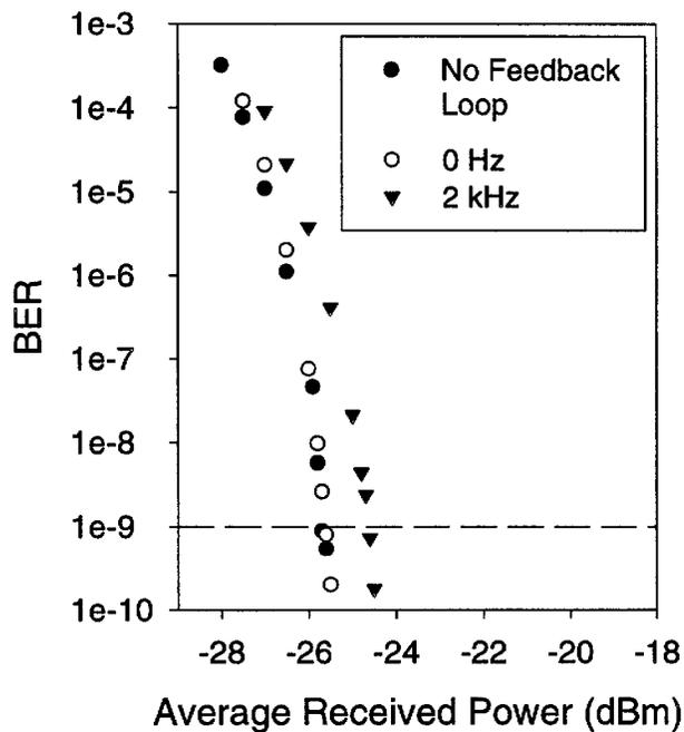
Fig. 5: BER performance of a 1-Gb/s  $2^{10}-1$  PRBS NRZ data on data wavelength at 1551 nm when the monitoring signal is sweeping at 2 kHz
