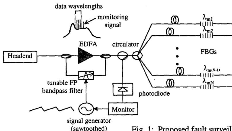
Fig. 1: Proposed fault surveillance scheme in an optically amplified branched network
