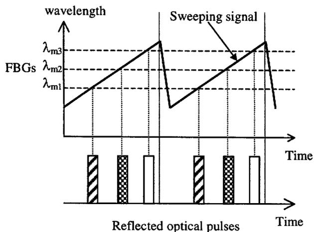
Fig. 2: Operation principle of the surveillance scheme
