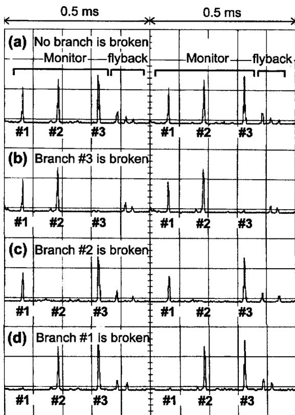
Fig. 4: Reflected optical pulse train at the monitoring module for different scenarios
