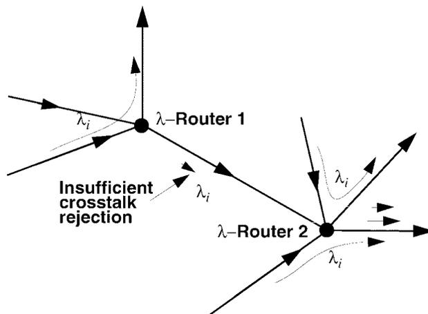
Fig. 1. Example of an optical network configuration that may induce homodyne crosstalk interference.
