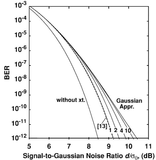
Fig. 2. BER as a function of signal-to-Gaussian noise ratio  $d/\sigma_0$  for a total crosstalk level of  $-25$  dB with different number of homodyne interferers and Gaussian approximation. The dash-line curve is the single-interferer result from [13].
