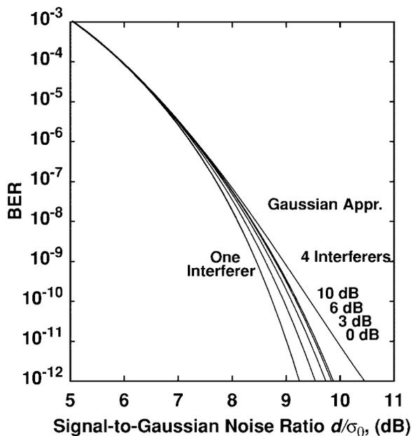
Fig. 4. BER as a function of signal-to-Gaussian noise ratio,  $d/\sigma_0$  for a total crosstalk level of  $-25$  dB. There are a total of four homodyne interferers with different crosstalk levels.
