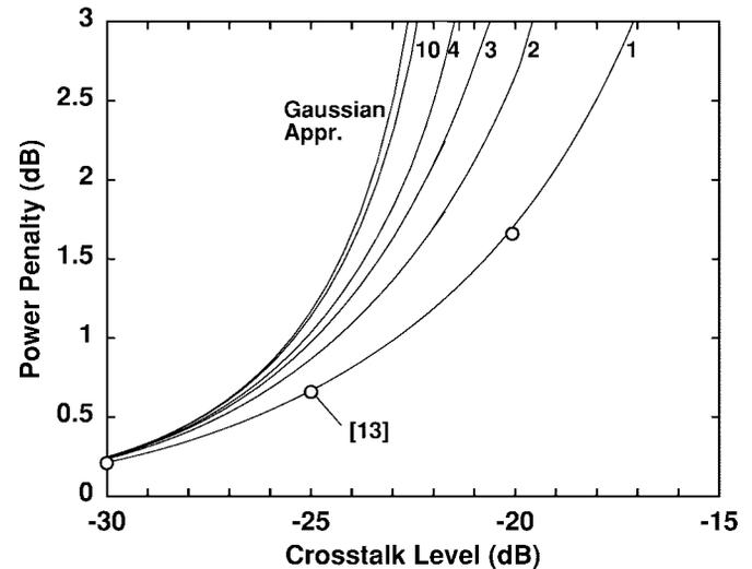
Fig. 3. Power penalty as a function of crosstalk level for different number of interferers and Gaussian approximation. The circles are power penalties from exact analysis for single interferer [13].
