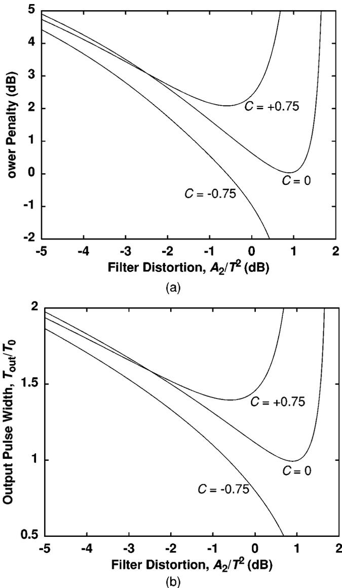
Fig. 3. (a) Power penalty and (b) pulsewidth as a function of normalized filter-distortion coefficient  $A_2/T^2$  for dispersive filter having  $\beta_2/T^2 = 0.1$ .
