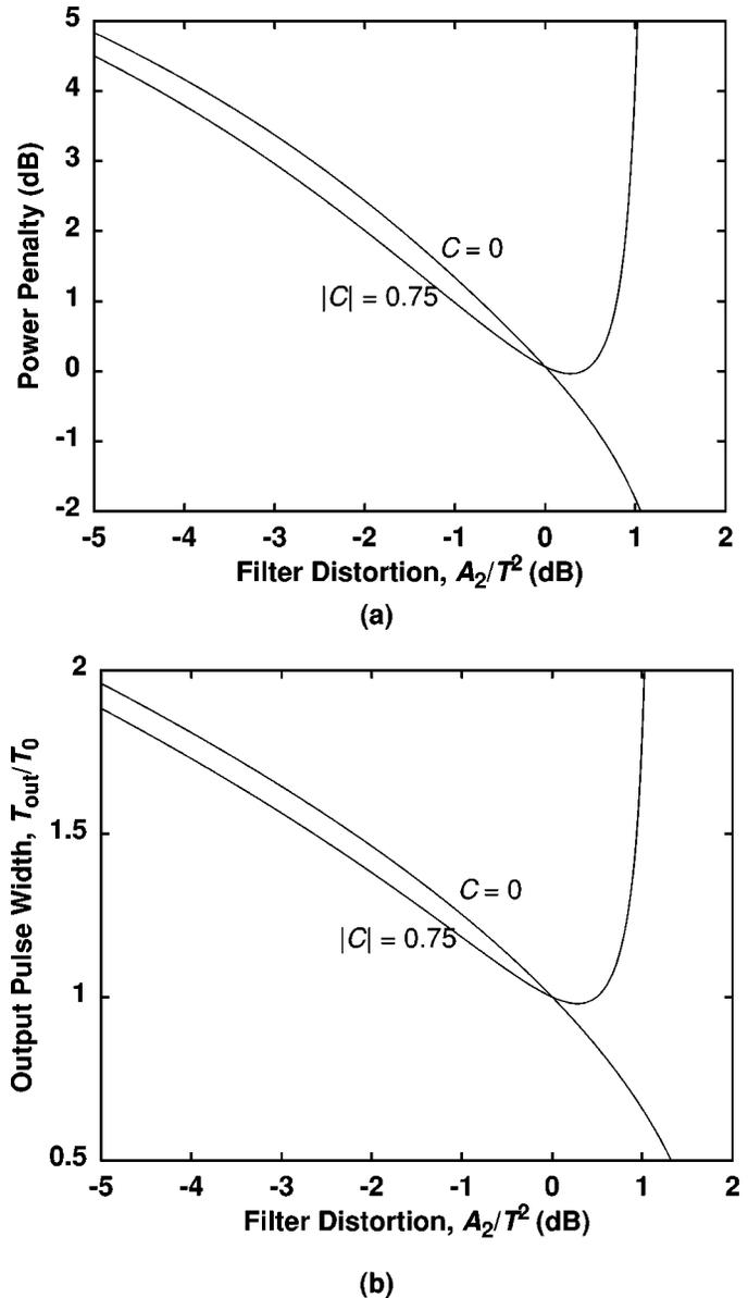
Fig. 2. (a) Power penalty and (b) pulsewidth as a function of normalized filter-distortion coefficient  $A_2/T^2$  for nondispersive filter with  $\beta_2 = 0$ .
