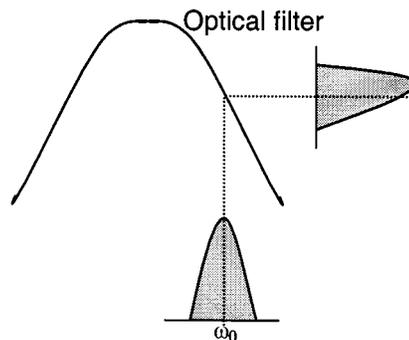
Fig. 1. Distortion induced by optical filtering.
