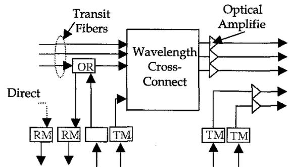
**Figure 1.** Proposed node architecture. TM is fixed-tuned transmitter module and RM is fixed-tuned receiver module, and OR is the optical relay.
