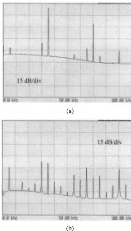
Fig. 4. Output from the electronic spectrum analyzer for the channel at  $\lambda_1$ : (a) without output analyzer; (b) with output analyzer.
