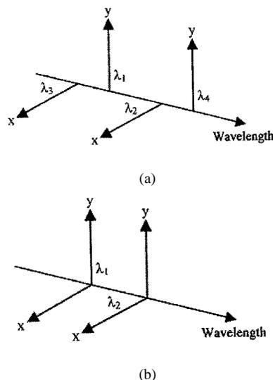
Fig. 1. Illustration of the polarimetric FWM process in (a) a birefringent fiber, (b) an SMF.
