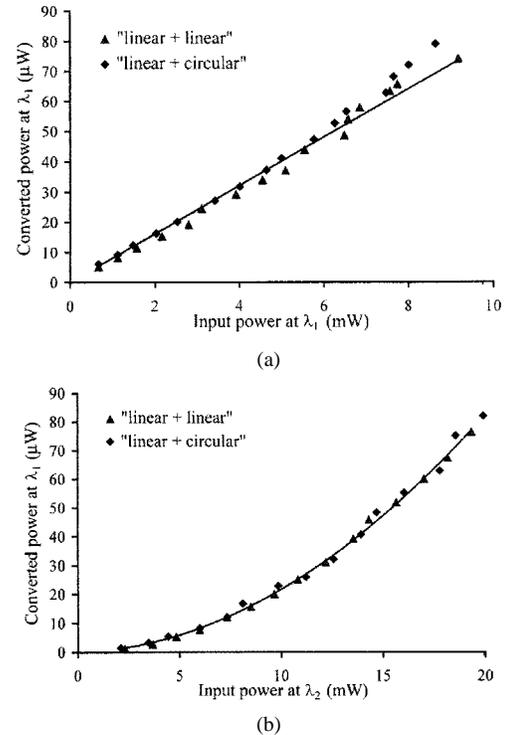
Fig. 3. Variation of the converted power at  $\lambda_1$  with (a) the input power at  $\lambda_1$  (with the input power at  $\lambda_2$  fixed at 19.9 mW) or (b) the input power at  $\lambda_2$  (with the input power at  $\lambda_1$  fixed at 8.6 mW) for two input polarization combinations.
