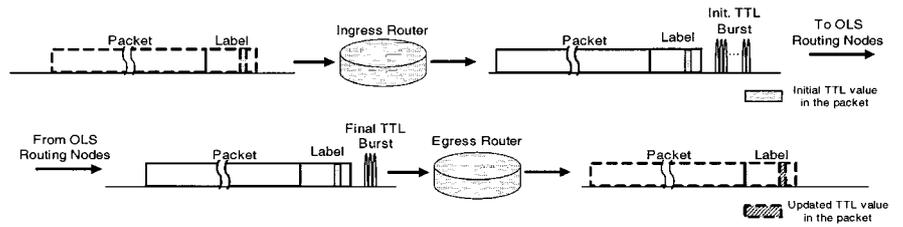
ThGG111 Fig. 1. Optical TTL field for OLS network routing loop control.
