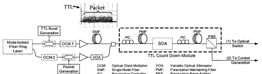
ThGG111 Fig. 3. TTL Countdown Demonstration (Inset: an example of packet with TTL pulses).
