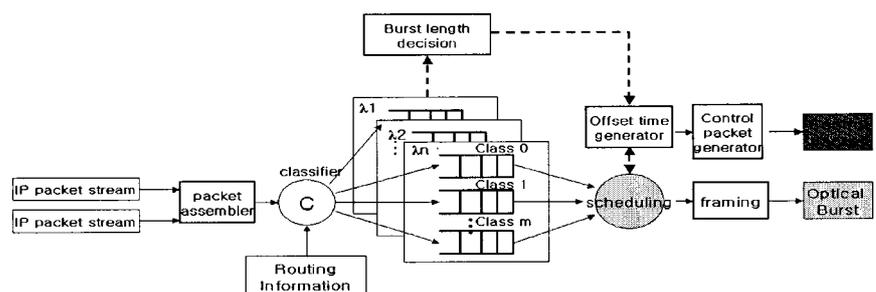
ThGG112 Fig. 1. Functional model of the ingress node in OBS networks.
