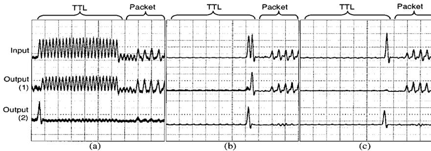
ThGG111 Fig. 4. Input pattern, output pattern at port (1) and output pattern at port (2) in Figure 3 for (a) 24, (b) 2 and (c) 1 pulse(s), respectively in the TTL burst (20 mV/div, 100 ps/div).
