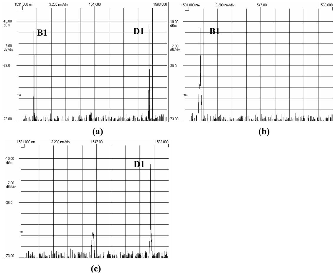
Fig. 4 (a) to (c): Optical spectra of the downstream signals at (a) output of OLT; (b) ONU#1; and (c) ONU#2.
