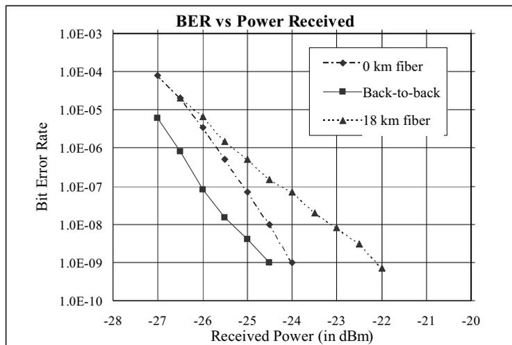
Fig. 5: BER performance of the 2.5Gb/s downstream wavelength
