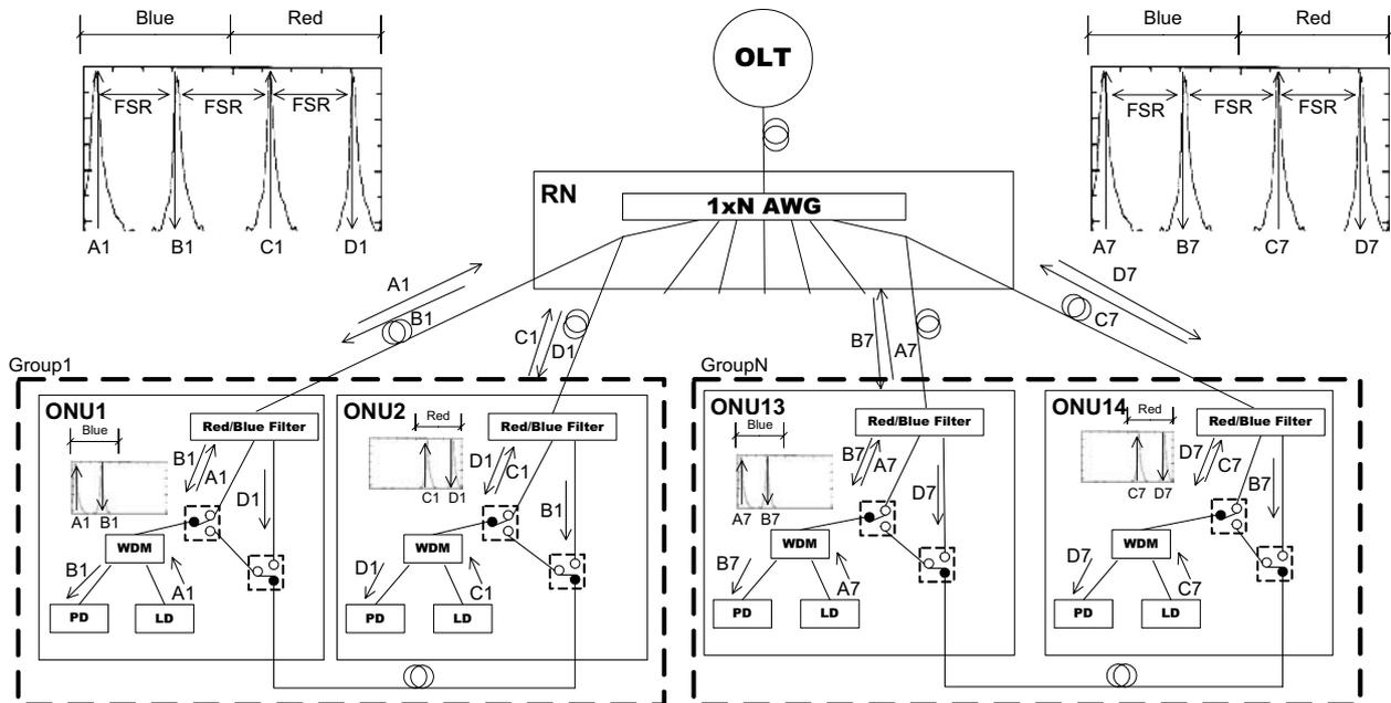
**Fig.1:** The proposed WDM-PON under normal operation. Insets show the corresponding optical spectra in the fiber links connecting the RN and the respective ONUs. (WDM: WDM Coupler; LD: laser; PD: photodiode)
