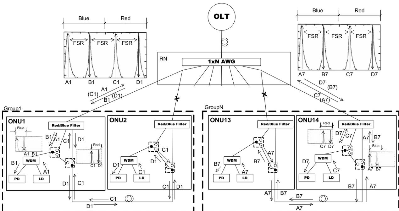
**Fig. 2:** The proposed WDM-PON when the fiber links connecting to ONU 2 and to ONU 13 are broken. The wavelength labels in brackets mean re-routed wavelengths.
