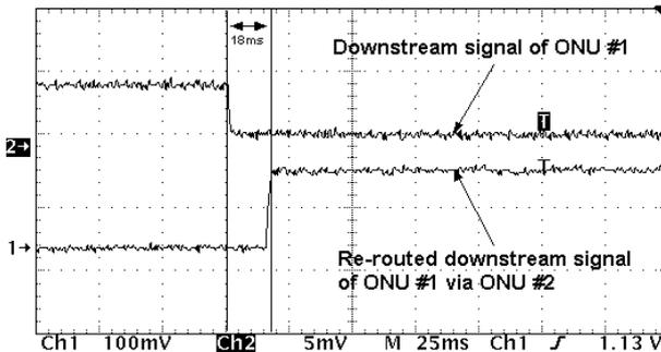
Fig. 4: Switching time measurement
