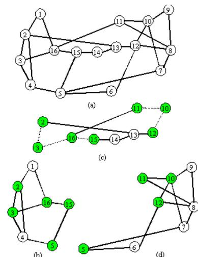
Fig. 1 (a) 16-node and 25-link NSFNET backbone. (b), (c), and (d) are three areas of (a). Working areas include only solid links. Protection areas include solid and dashed links. Node 5, 2, 3, 15, 16, 10, 11, and 12 are ABRs. The wavelengths on dashed links are permitted to be assigned only for protection sub-paths whose corresponding working sub-paths are in this working area.
